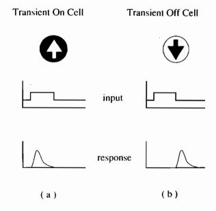
Figure 16. The transient cell filter consists of on-cells that react to input increments and off-cells that react to input decrements. (Reprinted, by permission, from Grossberg, 1991.)
