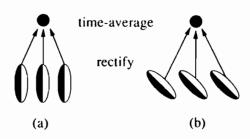
Figure 15. The sustained cell short-range filter combines several spatially contiguous receptive fields of like orientation via a spatial filter with a fixed directional preference. The orientation perpendicular to the direction is preferred, but nonorthogonal orientations can also be grouped in a prescribed direction. (Reprinted, with permission, from Grossberg, 1991.)
