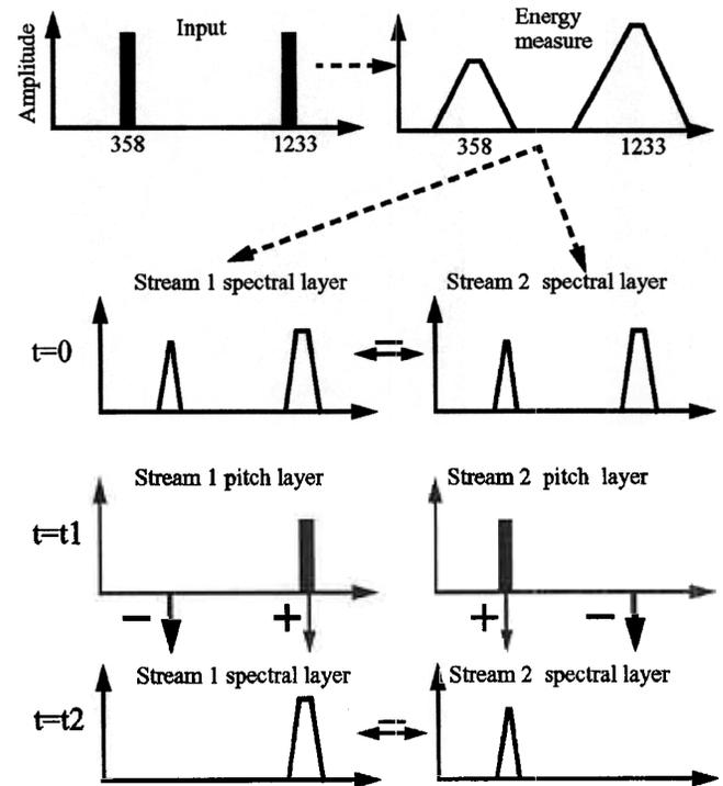
Fig. 14. Schematic of how the model segregates the two inharmonic tones into two different streams. See text for explanation.
