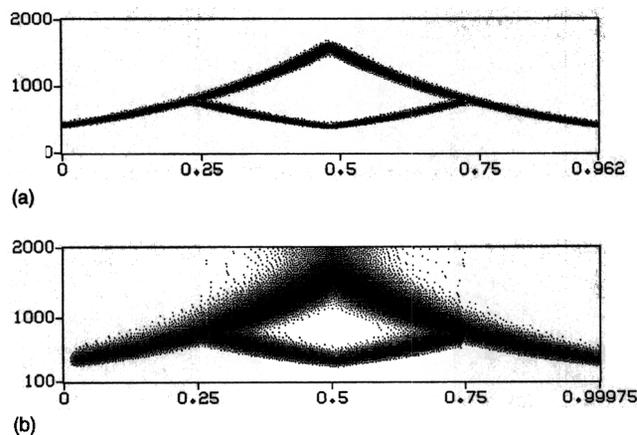
Fig. 28. (a) Spectrogram and (b) result of energy measure for the Steiger (1980) diamond stimulus.
