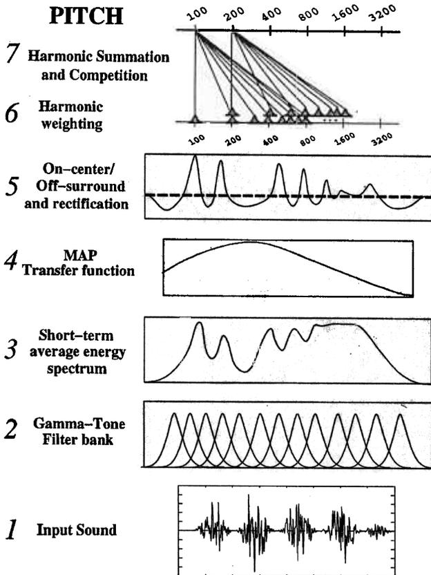
Fig. 9. Graphical representation of the SPINET model processing stages. [Reprinted with permission from Cohen, Grossberg, and Wyse (1995).]
