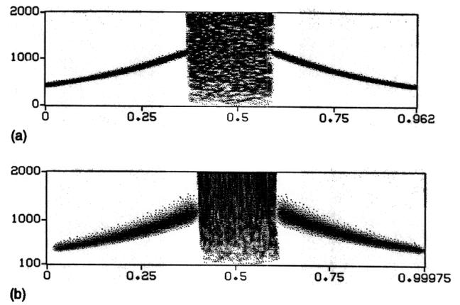
Fig. 20. (a) Spectrogram and (b) result of energy measure for the ramp stimulus.
