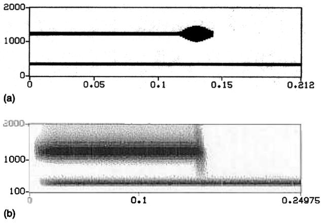
Fig. 12. (a) Spectrogram and (b) result of energy measure for the two tone stimulus.
