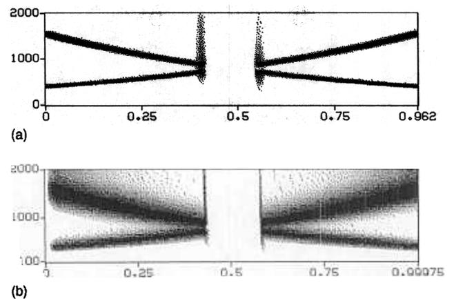
Fig. 24. (a) Spectrogram and (b) result of energy measure for the crossing glide stimulus with silence replacing the intersection point.
