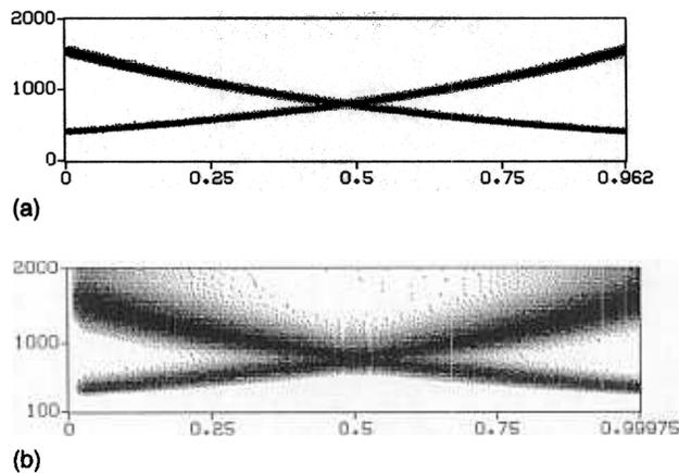
Fig. 22. (a) Spectrogram and (b) result of energy measure for the crossing glide stimulus.
