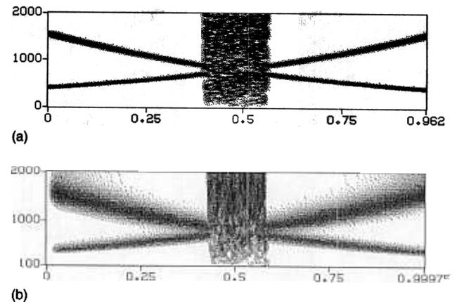
Fig. 26. (a) Spectrogram and (b) result of energy measure for the crossing glide stimulus with noise replacing the intersection point.
