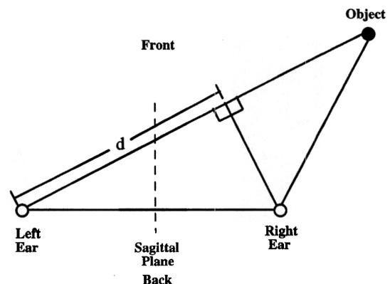
Fig. 32. Geometric representation of spatial lateralization using interaural timing differences (ITD).
