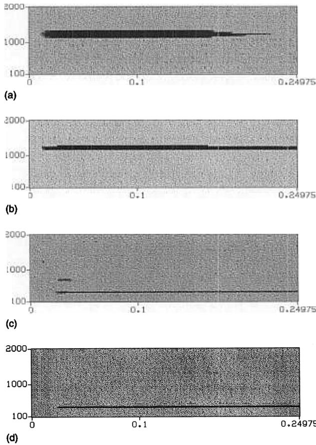
Fig. 13. Model results for the two tone stimulus. (a) spectral stream layer and (b) pitch stream layer for stream 1; and (c) spectral stream layer and (d) pitch stream layer for stream 2.
