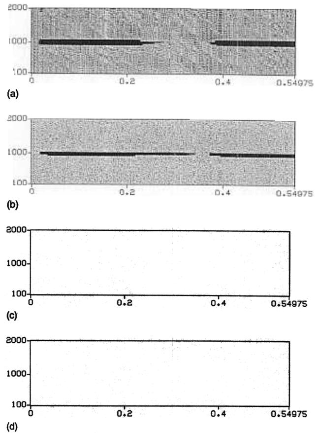
Fig. 16. Model results for the tone–silence–tone stimulus. (a) spectral stream layer and (b) pitch stream layer for stream 1; and (c) spectral stream layer and (d) pitch stream layer for stream 2.
