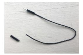
3. Strip the ends of the pin-equipped wires by clamping the wire strippers on the wire and then pull away from the wire. The rubber part should come off, and about 0.5 inches of wire should be exposed. These wires can be any color, as the ordering of the insertion of the pins for device output does not affect the output.
