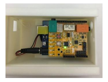
5. Plug the 3.5 mm male audio jack into the black relay pins as shown in the sequence below. Thread the pins of the plug, one at a time, through the smaller hole of the housing. Then insert the pins into the relay highlighted on the diagram below. It is labeled as "HHI" on the Muscle SpikerShield. This connection is what allows the switch to interface with existing AAC systems. It does not matter which colored wire plugs into each port of the relay pin.
