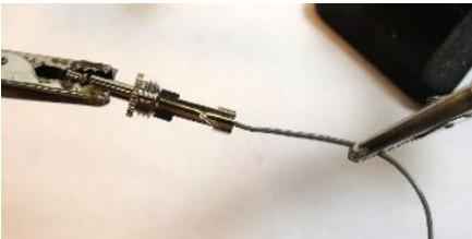
5. Solder the exposed pin-equipped wire with the pin of the audio jack together. Let cool.
