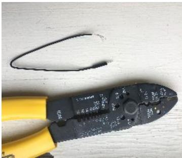
4. Place wires flat on a heat resistant surface, or hold them in place with soldering clamps, as shown. Position the exposed end of the pin-equipped wire with one of the metal pins of the audio jack and loop the wire through the hole. Ensure that the wire does not come in contact with the other pin or other stripped wire.
