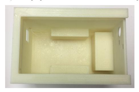
3. Place the battery into the housing as depicted in the photo below. The battery should lay lengthwise in the housing.
