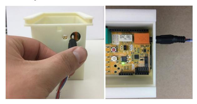
7. Slide the housing lid into the the grooves at the top of the base. Be sure to set the hook down so it catches the base of the housing.
