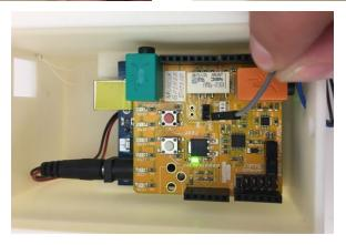
6. The Arduino may have shifted. It is alright to push it back into place such that the orange port is flush with the large hole. Insert the electrode snap plug into the orange port **through** the housing.
