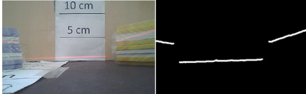
Fig. 9. Captured image (original) and successfully extracted laser lines.
