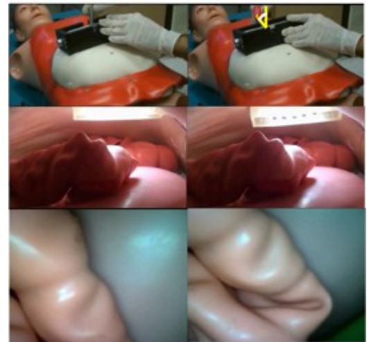
Fig. 13 Demonstration of tilting mechanism in a phantom test; on the top, external view; in the middle, view inside the abdomen of the internal unit; on the bottom, images acquired by one on-board camera.
