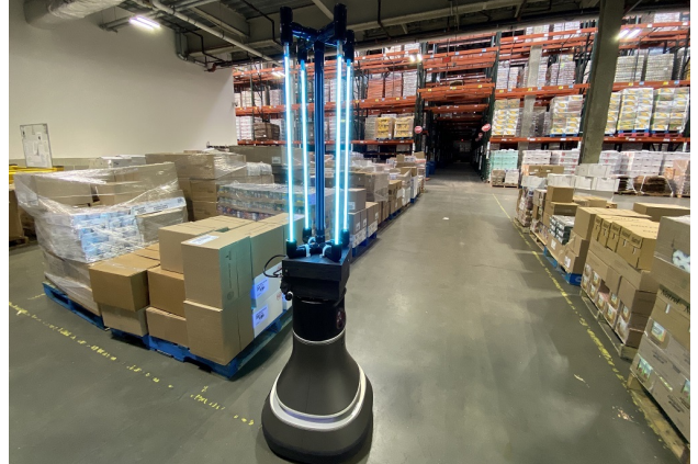
Fig. 1: Our UVC mobile disinfecting robot at The Greater Boston Food Bank. The robot performs nightly autonomous patrols of the aisles of pallets.
