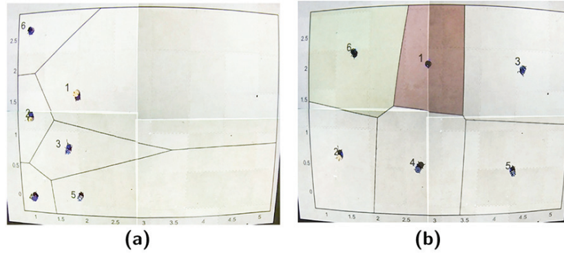
Fig. 20. In the initial configuration (a), note that all robots start off with equal weights. Robot 1 has the lowest health, but a relatively large cell, while robot 6 has a high health, but small cell. In the final configuration (b), the shading indicates the relative weights. Note that robot 1’s cell is now much smaller, and the red indicates its lower relative weight. Similarly, robot 6’s cell has increased in size, and the green indicates a relatively higher performance weight.
