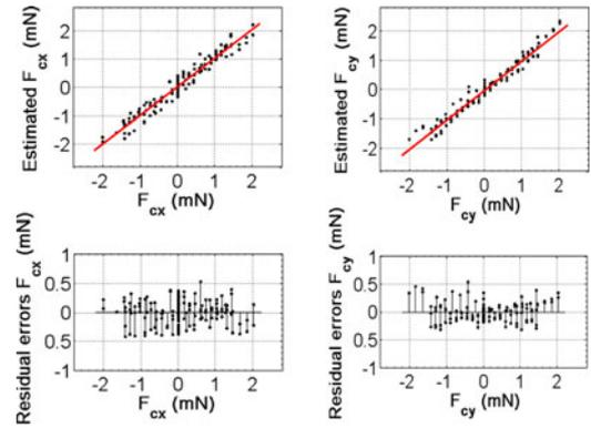
Fig. 15. Validation experiment results. On the top of the figure, force components  $F_{cx}$  and  $F_{cy}$ , estimated with the wavelength-to-force conversion matrix, versus the actual value of the force using linear fitting are reported. On the bottom of the figure, corresponding residual errors are shown.
