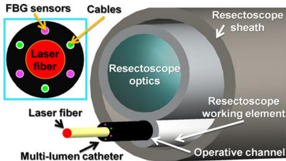
Fig. 3. Schematic overview of the ASTRO system design. In the inset, section of the multilumen catheter integrating the laser fiber, the FBG sensors (in pink) and actuation cables (in green) is shown.
