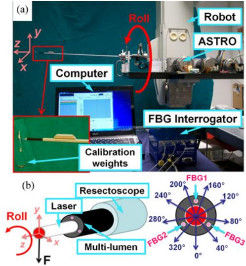
Fig. 12. Calibration setup: (a) picture of the calibration setup showing the ASTRO system mounted on the robot, the FBG interrogator, the computer and calibration weights, (b) schematic representation of the system orientation during calibration ( $40^\circ$  rolling angles). Calibration chamber is not shown in the picture.
