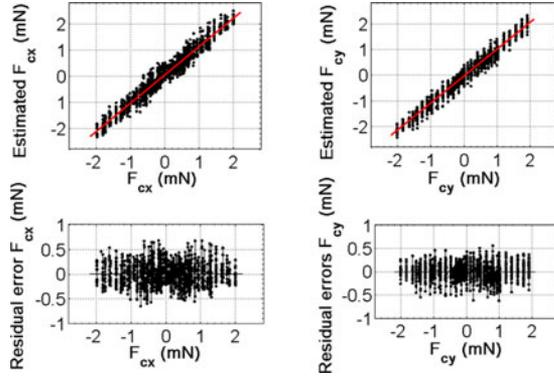
Fig. 13. Calibration results. On the top of the figure, force components  $F_{cx}$  and  $F_{cy}$ , estimated with the wavelength-to-force conversion matrix, versus the actual value of the force using linear fitting are reported. On the bottom of the figure, corresponding residual errors are shown.
