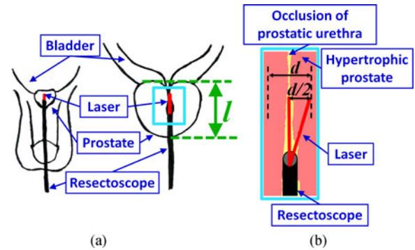
Fig. 2. Laser tip steering: definition of requirements for the actuation unit: (a) overview of the laser procedure for BPH; (b) close view of the laser in the prostatic urethra.
