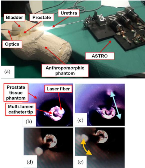
Fig. 11. Actuation assessment test with the anthropomorphic phantom: (a) experimental setup, (b) and (c) approaching phases of the laser tip to the tissue phantom, (d) and (e) slicing phases of the laser tip on the tissue phantom. During experiments, optics is inserted in the phantom so as to point towards the front of the ASTRO system.
