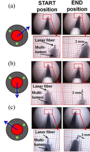
Fig. 10. Actuation assessment. The direction of steering, for each test, is schematically shown in the left part, respectively, in (a), (b), and (c). The laser tip steering, recorded through the resectoscope optics, is shown in the right part of the figures. A close view of the laser tip steering is shown in the bottom of each figure.
