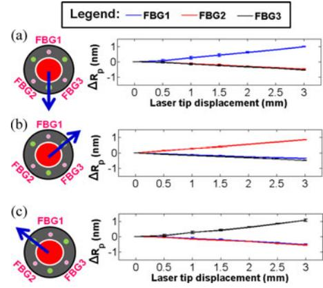
Fig. 14. Calibration results of the ASTRO system under steering (no-contact-force condition). The three sensors differential signals, for the three steering directions are shown. For each graph (a), (b), and (c), the three components of the vector  $\Delta R_p$  are shown as scalars. The steering directions are shown in the scheme on the left: cables are in green, FBG sensors are in pink.
