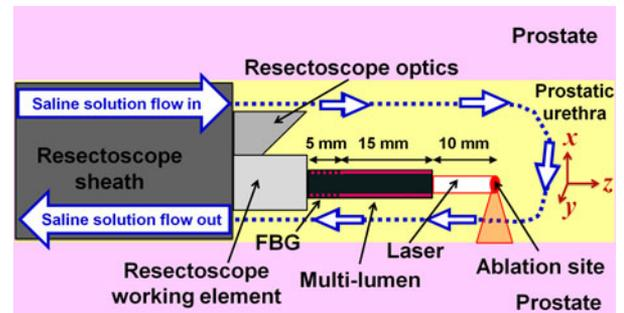
Fig. 7. Schematic representation of the ASTRO sensing system design: FBG positioning within the ASTRO system (FBG sensors are integrated inside the multi-lumen catheter and two of them are visualized in the picture for clarity).
