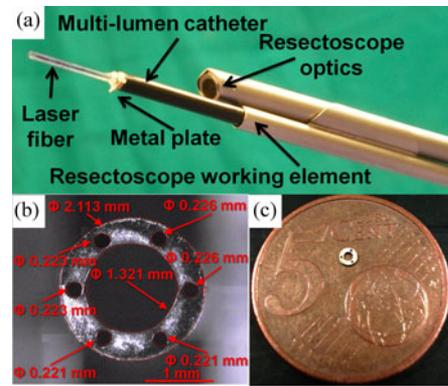
Fig. 4. Multilumen catheter: (a) tip of the ASTRO system, with the multilumen catheter inserted in the resectoscope, (b) picture of the multilumen section at the optical microscope, (c) metal plate to fix the cables on a 5 cent euro coin.
