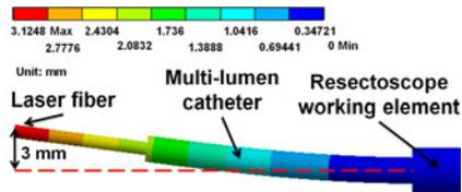
Fig. 5. Finite-element results: computation of total deformation in millimeter of the system when a 12-N pulling force on the cable is applied.
