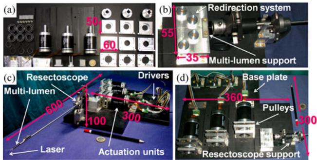
Fig. 6. Actuation unit of the ASTRO system: (a) components of the actuation mechanism, (b) closeup view of multi-lumen support and redirection system of the cables, (c) assembled actuation system, (d) closeup view of the pulleys.
