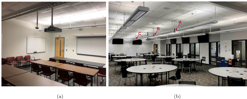
Fig. 2. (a) 500 ft 2 classroom monitored by a single camera mounted 8-1/2 ft above the floor; (b) 2,000 ft 2 studio-style classroom monitored by 3 cameras mounted 10 ft above the floor. The distance between cameras A and B is 121 in, and between cameras B and C it is 248 in. All cameras shown are Axis M3057-PLVE (3,072×2,048 pixels, 185° lens).
