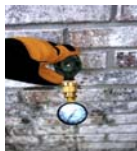
Water pressure gauge, Florida
