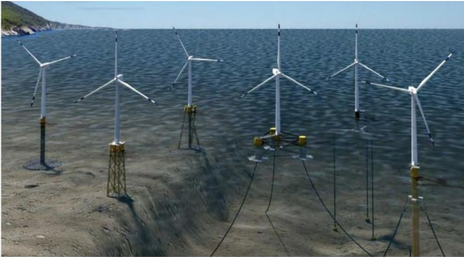
From left to right: a monopile, jacket, twisted tripod, floating semi-submersible, floating tension leg platform and floating spar.
