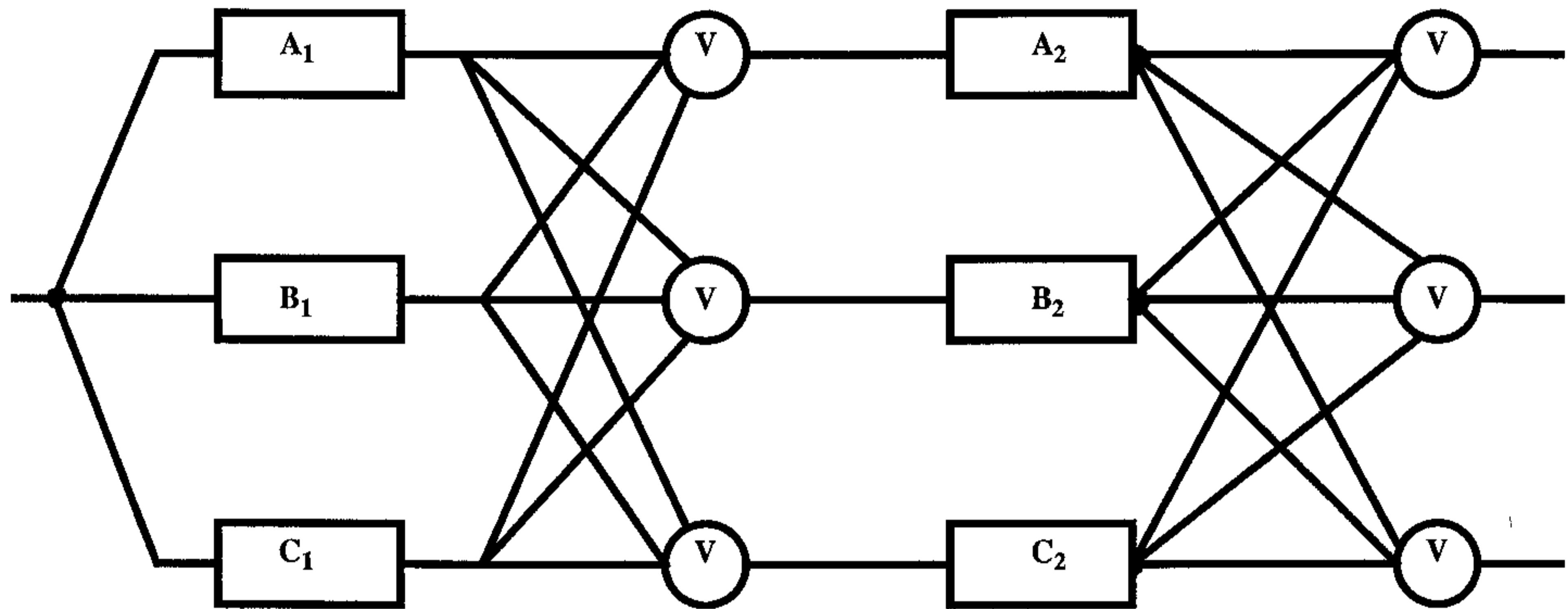
For the fault - free case :  $A_1 = B_1 = C_1, A_2 = B_2 = C_2$
