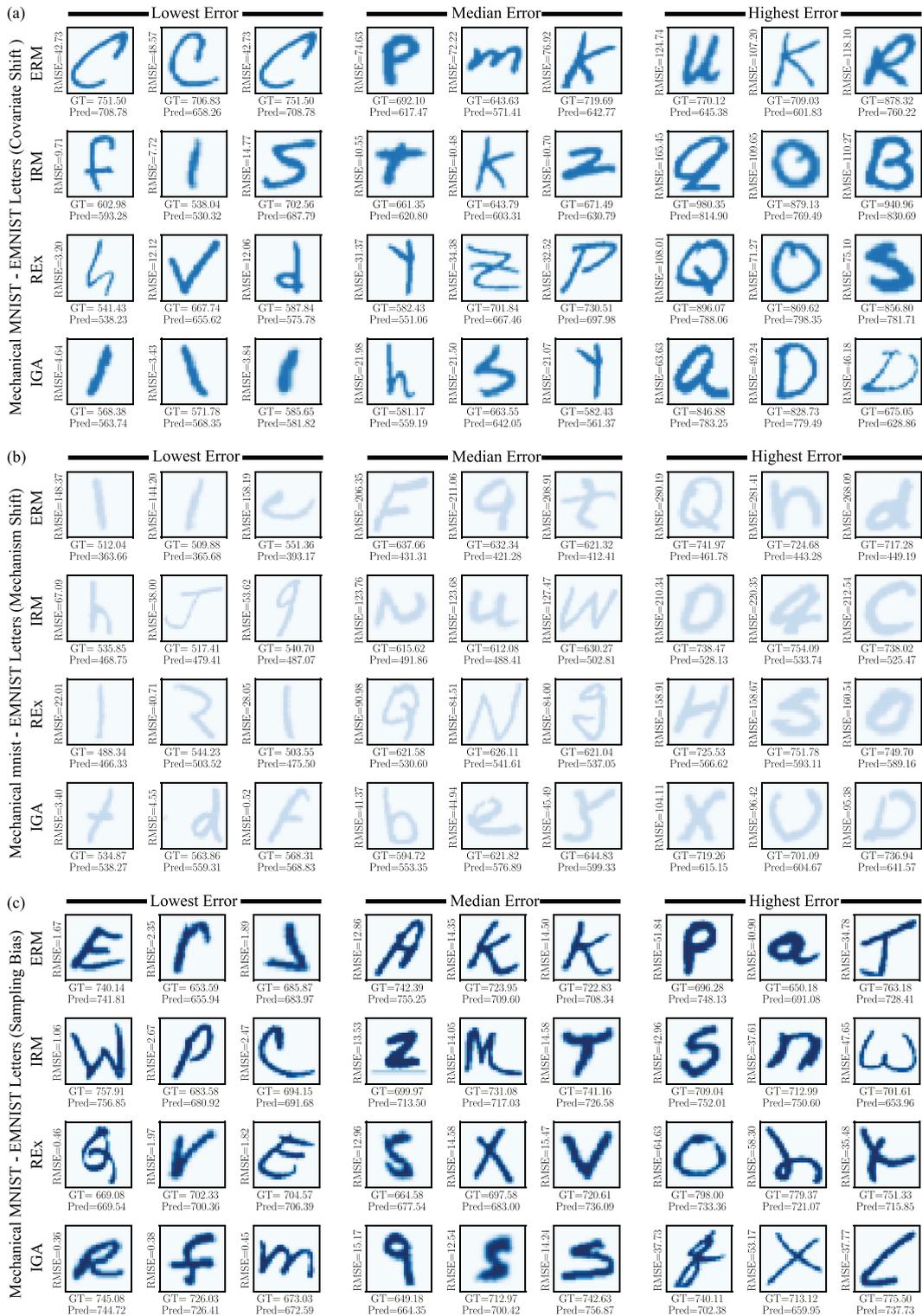
**Fig. 19.** The sampled cases of three groups: lowest error (bottom 10% RMSE), median error (45% - 55% RMSE) and highest error (top 10% RMSE) from the Mechanical MNIST - EMNIST Letters collection and the corresponding ground truth and prediction of the change in strain energy. For each OOD dataset (a) Covariate Shift (b) Mechanism Shift and (c) Sampling Bias, the error (RMSE) is calculated and sorted based on the predicted value given by LeNet model on ERM, IRM, REX, and IGA respectively.
