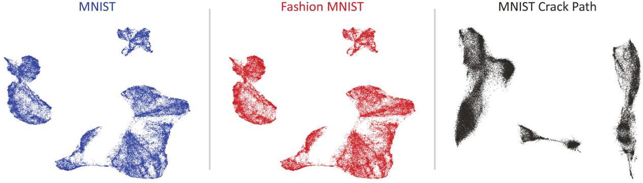
Fig. 6. Visualization of the input parameter space for the Mechanical MNIST dataset [48], the Mechanical MNIST Fashion dataset [47], and the Mechanical MNIST Crack Path dataset [52] using the UMAP algorithm with default parameters ( n\_neighbors=15 , min\_dist=0.1 , n\_components=2 , metric="euclidean" ) [82].
