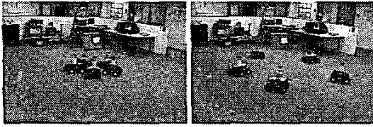
Figure 3: Initial and final configuration in an expansion maneuver - control of shape while pose is preserved
