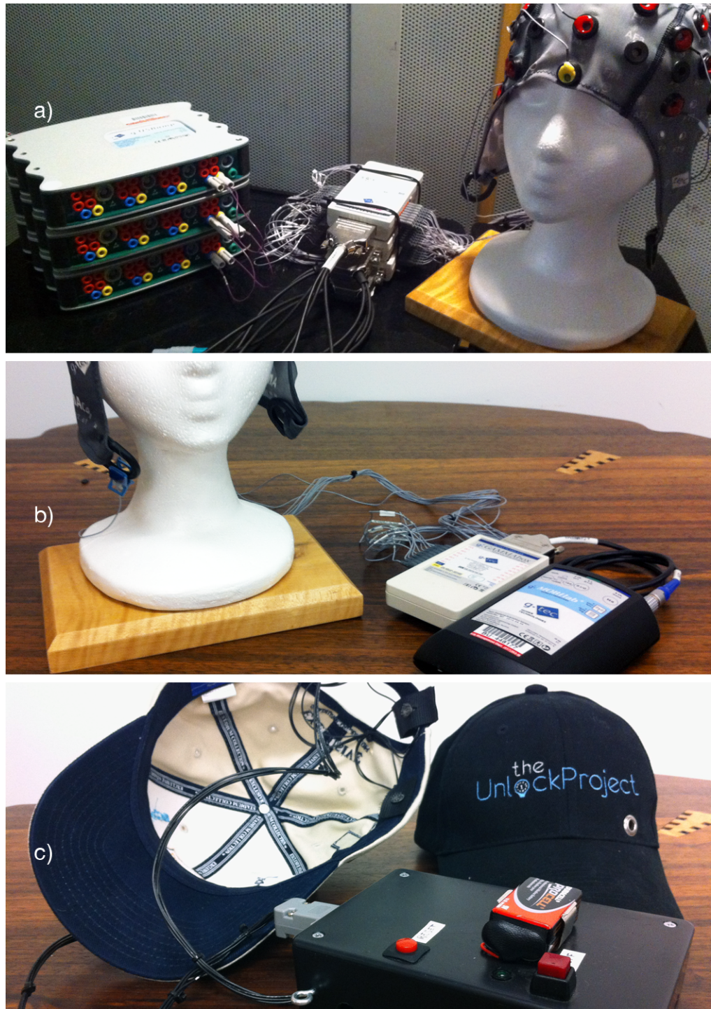
Figure 2-3. a) g.Tec research BCI setup; b) g.MOBilab+ mobile BCI setup; c) Unlock Project custom dry electrode setup.
