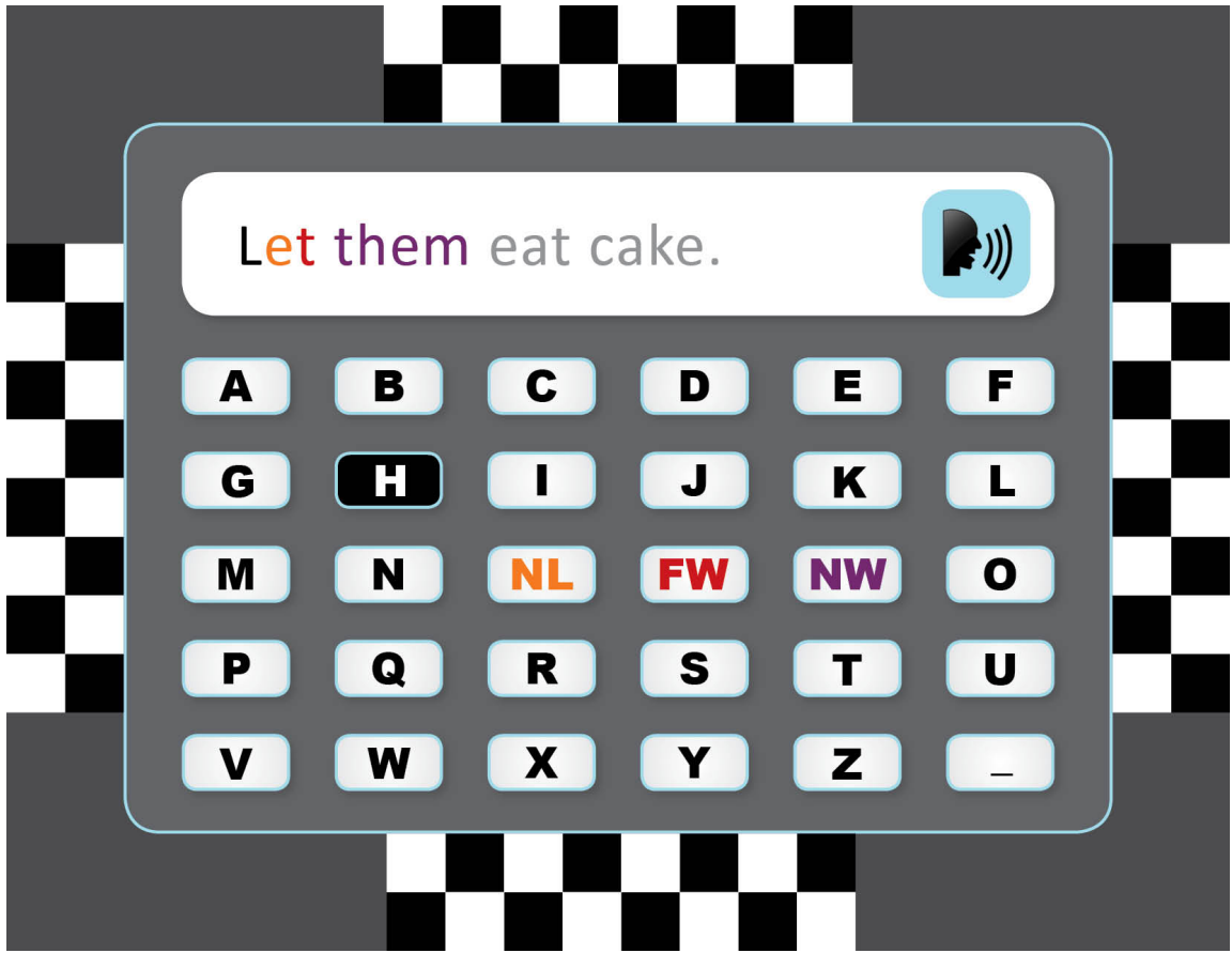
Figure 5-7. The ContextSpeak communication app GUI for an SSVEP-based BCI. The current cursor position is shown with a black key and white text.
