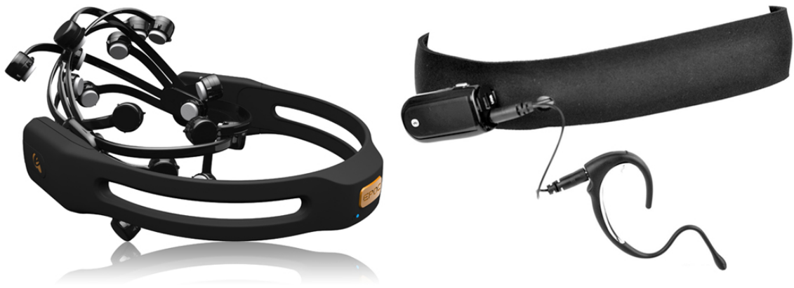
Figure 2-2. The Emotiv Epoc EEG headset (left) and NeuroSky MindBand EEG sensor band (right).
