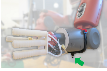
Fig. 5: A mechanical momentary switch affixed to the bottom of Baxter's arm precisely determines when the arm begins moving. This feedback onset time is vital for reliable EEG classification.
