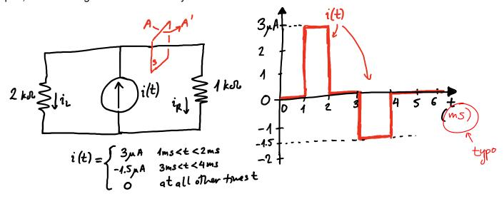
(a) [5] Find currents  $i_R$  and  $i_L$  for all times t shown in the plot, and sketch a plot of the two currents vs. time for t = 0 to 6 ms.
