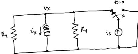
a switch is toggled at time t=0 as shown. Here,  $i \le 1$  mA, R1 = 2kW, R2 = 2kW, and the inductor inductance value is  $L = 1\mu H$ .
