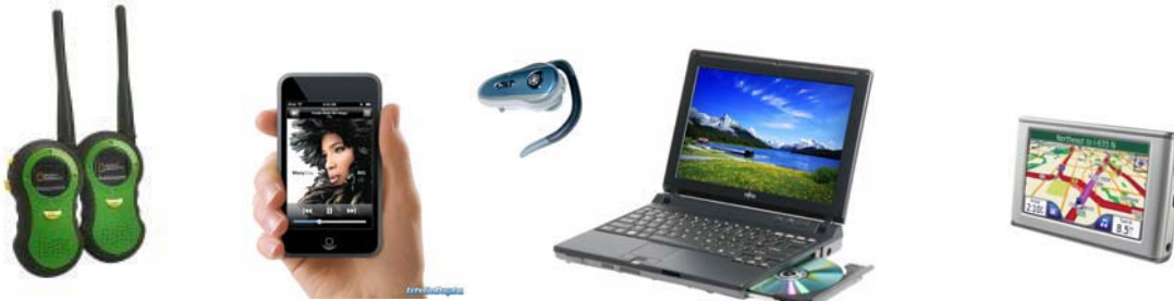
Common devices requires sources of low-voltage dc power
