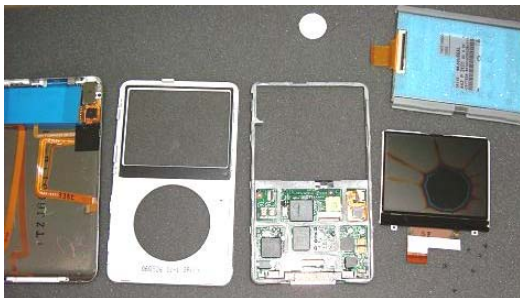
A reverse-engineered iPod. Note the broken screen on the right: a casualty of the disassembly process.
