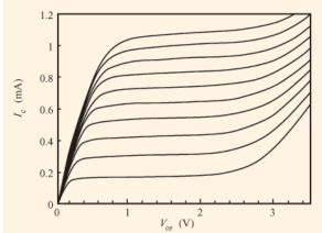
Here, several representative values of  $i_{\rm B}$  are chosen for the plot, with the understanding that the  $i_{\rm C}$ - $v_{\rm CE}$  curve varies continuously between the curves that are chosen for plotting.
