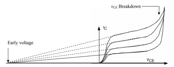
As you have may have learned in lecture, and as is discussed in the text, extending the transistor's constant-current curves into the left-hand quadrant causes them to intersect the voltage axis at the so-called *Early voltage*. This feature is shown in the above plot. (Note that the Early-voltage parameter is named after a person, not a time.). The breakdown value of  $v_{CE}$  is less definitive, because breakdown does not occur abruptly with increasing  $v_{CE}$ .
