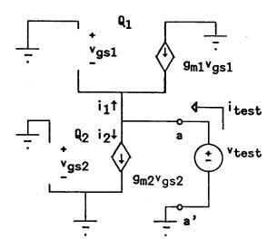
The vtest source fixes  $v_{gs1}$  to the value  $-v_{test}$ , so that  $i_1 = -g_{m1}v_{gs1} = g_{m1}v_{test}$ . Meanwhile, both sides of  $v_{gs2}$  are grounded, so that  $v_{gs2} = 0$  and  $i_2 = g_{m2}v_{gs2} = 0$ . The current leaving the  $v_{test}$  source is thus equal to  $i_{test} = i_1 + i_2 = g_{m1}v_{test}$ .
