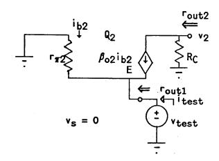
From the test circuit shown above,  $i_{b2}$  becomes  $-v_{test}/r_{\pi 2}$ , so that  $i_{test}$  becomes
