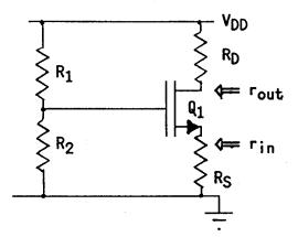
8.8 In the circuit shown below, the gate of  $Q_1$  is driven by a small-signal voltage source  $v_s$ . Find the small-signal gain  $v_{out}/v_s$  if  $Q_1$  is biased in the constant-current region
