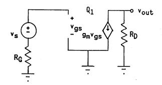
In this incremental circuit, the voltage v<sub>qs</sub> is equal to v<sub>s</sub>. Note that no current flows through Rg, hence the voltage drop across RG is zero. The dependent current source pulls a current  $g_{m}v_{qs}$  up from ground through RD, so that the small-signal output becomes
