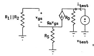
In this case, KVL taken around the loop containing v<sub>gs</sub> yields
