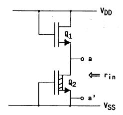
8.3 Consider the MOSFET current mirror shown below, in which  $I_1$  is replicated as  $I_2$ . Find an expression for the small-signal input resistance  $r_{th}$  seen at the drain terminal of  $\mathbb{Q}_2$ .
