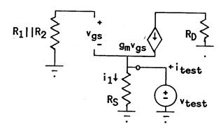
The applied source fixes  $v_{gs}$  to the value -vtest, so that itest, which has two components, becomes
