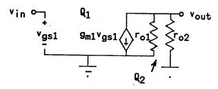
By inspection,  $v_{gs1} = v_{in}$ . The dependent source pulls current up through the parallel combination  $v_{o1}||v_{o2}$ , so that the output becomes  $v_{out} = -g_{m1}(v_{o1}||v_{o2}) v_{in}$
