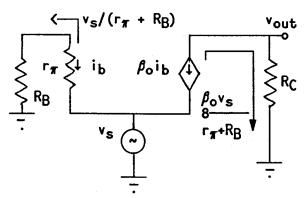
The voltage drop across  $r_{\pi}$  (defined as positive from the top of  $r_{\pi}$  to the bottom) is equal to  $-v_s$ . Hence  $i_b = -v_s/(r_{\pi} + R_B)$ . This current is replicated as  $\beta_{oib}$  by the dependent source of the incremental model, so that a current  $\beta_{ov_s}/(r_{\pi} + R_B)$  flows down into  $R_C$  in the direction shown.
