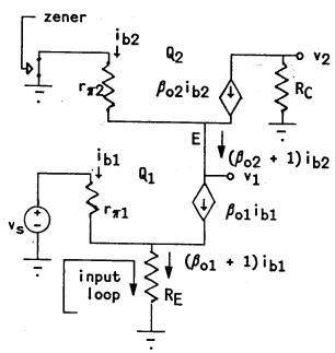
a) Find the small-signal gains measured at  $v_1$  and  $v_2$ . From KVL around the input loop,
