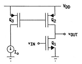
8.14 Find the small-signal output of the CMOS amplifier shown below. Assume that  $v_{IN}$  contains a dc bias component that biases both  $Q_1$  and  $Q_2$  into the constant current region.
