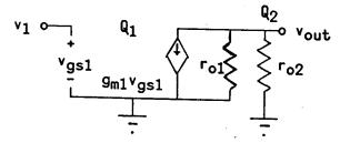
Note that  $r_{o1}$  and  $r_{o2}$  must be included in the model, because no smaller resistances appear in parallel. This feature is characteristic of many CMOS circuits.
