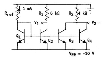
7.12 In the Widlar source shown below, find the bias current  $I_o$  at room temperature ( $\eta V_T = 25$  mV) if  $V_f \simeq 0.7$  V
