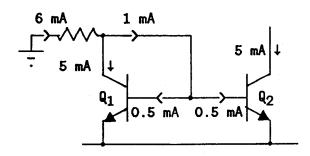
b) The following circuit configuration provides a buffer to the bases of  $\mathbb{Q}_1$  and  $\mathbb{Q}_2$ .
