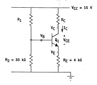
Repeat the previous problem if the BJT is replaced by an n-channel MOSFET with K = 0.1 mA/V<sup>2</sup> and V<sub>TR</sub> = 0.5 V. In this case, let R<sub>2</sub> = 1 M $\Omega$ . The current through the device is to be set to I<sub>D</sub> = 1.7 mA with V<sub>DS</sub> = 6 V.
