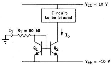
7.11 In the following current mirror all transistors are matched. Find  $R_{ref}$ ,  $V_1$ , and  $V_2$  if  $V_f \simeq 0.7$  V. Neglect base currents with respect to collector currents.
