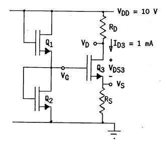
7.8 Consider the depletion-mode MOSFET circuit shown below. Both devices have parameters K = 0.2 mA/V<sup>2</sup> and  $V_{TR}$  = -2 V. Find the bias current ID and the voltages  $v_{OUT}$ ,  $V_{DS1}$  and  $V_{DS2}$ .
