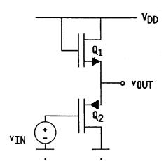
6.15 Find the transfer characteristic of the JFET circuit shown below. The devices have the same values of  $\mbox{Vp}$  and  $\mbox{I}_{DSS}$ .
