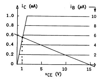
With R<sub>C</sub> = 25 k $\Omega$ , the intercepts of the load line are V<sub>CC</sub> = 15 V (open circuit voltage of the Thevenin circuit formed by V<sub>CC</sub> and R<sub>C</sub>) and V<sub>CC</sub>/R<sub>C</sub> = 0.6 mA (short circuit current of the Thevenin circuit).
