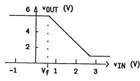
Note that  $v_{OUT}$  remains fixed at  $V_{CC}$  until  $v_{IN}$  exceeds the BJT "threshold" voltage  $V_f$ . Similarly, for values of
