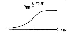
6.10 Determine the general form of the voltage transfer characteristic of the NMOS/PMOS (CMOS) circuit shown below
