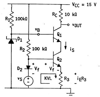
In this circuit, the large resistance  $R_2$  forward-biases  $D_2$  by forcing a small current through the diode and into the  $v_S$  source. The voltage drop across  $D_2$ , which is approximately equal to  $V_f$ , is used to overcome the base-emitter voltage drop of  $\mathbb{Q}_2$ . Applying KVL to the base loop of  $\mathbb{Q}_2$  yields
