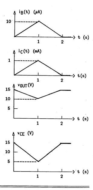
iB will again be equal to ig. In this case, however, the larger values of RC and RE will cause a larger proportional drop in vout and vCE for the same increase in ic. Thus Q1 will reach its saturation point, with vCE = Vsat, before the peak of ig is reached. The exact values of ic and vCE at saturation can be found by plotting the load line of the voltage VCC and total resistance (RC + RE) over the BJT v-i characteristics:
