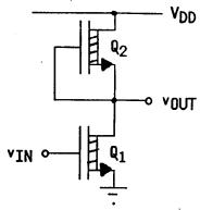
Note that  $Q_2$  has its gate connected to its source, so that  $v_{GS2}=0$ . This connection allows  $i_{D2}$  to be nonzero for all values of  $v_{DS2}$ . The exact value of  $v_{DS2}$  is determined by the  $v_{GS}=0$  v-i characteristic of  $Q_2$ . The current through  $Q_2$  is set by  $Q_1$ .
