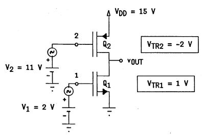
6.17 Consider the CMOS circuit described in Prob 6.16. Suppose that the two inputs are connected together and driven by a common input source vIN. Make a qualitative sketch of the resulting vIN-vour transfer characteristic.
