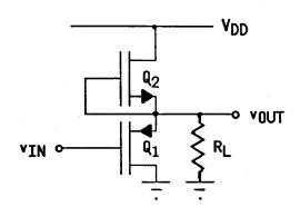
A depletion-mode p-channel device has a positive  $V_{TR}$ , yielding a positive turn-on value of  $v_{IN}$ . This condition is compatible with the indicated transfer characteristic.
