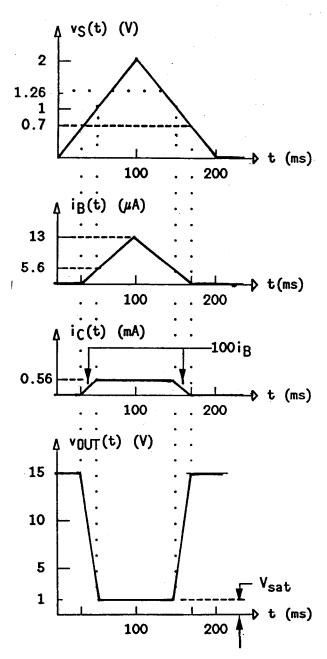
6.3 The value of V<sub>f</sub> for the baseemitter junction of the BJT is irrelevant to this problem. The is(t) forces its current source current into the base of Q1 regardless of the value of vBE. voltage across the is source adjusts itself to be whatever value of vBE is required for the established ig.
