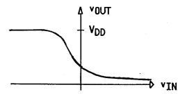
6.9 Using only n-channel and p-channel depletion-mode MOSFETs, design a CMOS circuit whose voltage transfer characteristic has the basic form shown below. Note that  $v_{OUT}$  is equal to  $V_{DD}/2$  at  $v_{IN}=0$ . The circuit drives a load resistance  $R_{L}$ .
