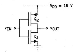
For  $v_{IN}$  >  $v_{TRN}$ ,  $v_{GS1}$  will exceed the threshold voltage of  $Q_1$ , causing the n-channel device to conduct and  $v_{OUT}$  to be forced toward ground. Over this region of operation,  $Q_2$  will function as the pullup load to  $Q_1$ .
