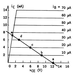
The transfer characteristic of the circuit, found by plotting the points (a) - (e), is shown below. For  $v_{IN} < V_f$ , iB is zero (cutoff), so that iC = 0 and  $v_{OUT} = V_{CC} = 12 \text{ V}$ . For  $v_{IN} \simeq 4.2 \text{ V}$  (iB  $\simeq 36 \mu$ A), the BJT enters saturation, and  $v_{OUT} \simeq 1 \text{ V}$ .
