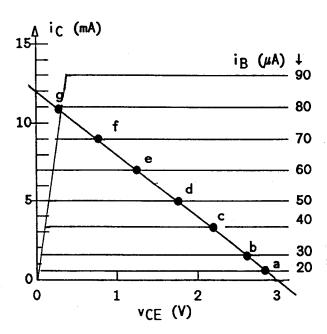
The base current  $i_B$  corresponds to the input current  $i_{IN}$ . The points of intersection of the load line with the various BJT v-i curves can thus be used to plot  $v_{OUT}$  versus  $i_{IN}$ :
