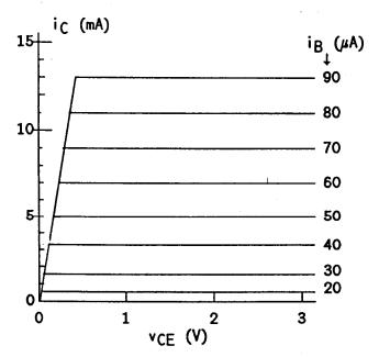
5.12 The BJT of Prob. 5.11 is installed in the circuit shown below. Use the graphical technique to plot  $v_{OUT}$  versus  $i_{TN}$ .
