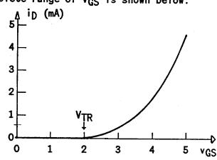
indicated circuit, plot the load line imposed by  $V_{DD}$  and  $R_D$  on the  $v_{DS}$ -ip v-i characteristic of  $Q_1$ . The  $v_{QS}$ -ip plot found in Prob. 5.8 can be used because the gate of  $Q_1$  is connected to its drain, so that  $v_{QS} = v_{DS}$ . In essence,  $Q_1$  functions as a two-terminal square-law device. From the plot shown, ip  $\simeq 0.75$  mA;  $v_{QS} \simeq 3.2$  V.
