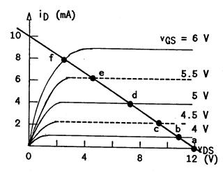
The resulting transfer characteristic can be found by plotting the points (a) - (f), as shown below. Note that for  $v_{IN} < v_{TR} = 3$  V,  $i_D = 0$  and  $v_{OUT} = v_{DD} = 12$  V.
