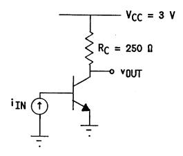
5.13 The BJT in the following circuit has a  $\beta_F$  of 100. Find  $V_B$ ,  $V_C$ , and  $V_E$ .
