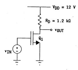
5.5 A BJT with the indicated v-i characteristics is connected to the circuit shown. Using graphical techniques, plot the  $v_{IN}$ - $v_{OUT}$  transfer characteristic.
