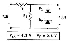
can be realized by a circuit in which the output is clamped in both the positive and negative directions. The following two circuits will accomplish the desired objective. Other solutions are possible. For each of the diodes shown, V<sub>f</sub> = 0.7 V.
