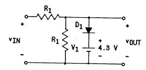
For  $v_{IN} > v_1 + v_f$ , the diode will conduct and clamp  $v_{0UT}$  to the value  $v_1 + v_f$ . The desired value of this
