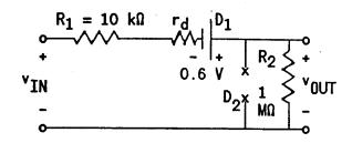
For  $v_{IN}$  >  $-v_f$ ,  $D_1$  becomes reverse biased, effectively disconnecting the  $v_{OUT}$  terminals from the rest of the circuit. Under these conditions,  $v_{OUT} = 0$ . Note that  $D_2$  is not forward biased for any value of  $v_{IN}$ .
