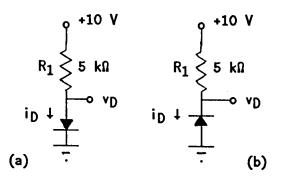
4.4 Find ip and  $v_R$  in the following circuits. For each diode,  $V_f = 0.5 \text{ V}$ .
