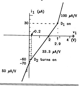
that it will tend to force  $D_1$  into reverse breakdown. The latter condition will be established if the reverse current  $i_2$  into the zener remains positive. If the zener is assumed to be in reverse breakdown, with  $v_{OUT} = V_{ZK}$ ,  $i_1$  will be given by
