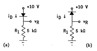
4.5 Find the diode voltage and current in the following circuit.  $D_1$  has a turn-on voltage of  $V_f = 0.5 \text{ V}$ .
