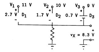
By KVL,  $v_X = V_3 - V_f = 9 \text{ V} - 0.7 \text{ V} = 8.3 \text{ V}$ . This condition would appear to result in diode voltages
