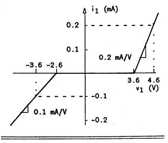
4.13 Consider the circuit with neither diode forward biased (both diodes set to open circuits). Under such conditions, the current becomes
