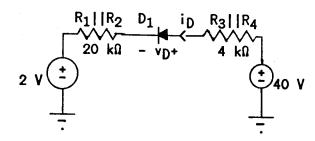
In this case the voltage on the right side of the diode is larger than the voltage on the left side;  $D_1$  becomes forward biased with  $v_D = 0.5 \text{ V}$  and
