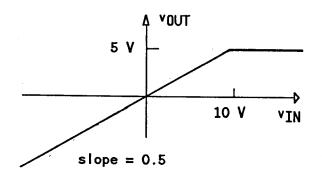
4.19 Design a limiter circuit that has the following voltage transfer characteristic:
