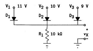
4.10 Plot  $i_1$  versus  $v_1$  for the circuit shown below if each diode has a  $V_f$  of 0.6 V:
