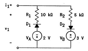
4.13 Plot the i-v relation of the circuit shown below if each diode has a turn-on voltage of  $V_f = 0.6 \text{ V}$ :
