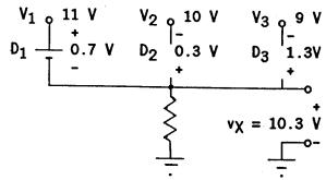
With  $D_1$  forward biased, diodes  $D_2$  and  $D_3$  are reverse-biased by voltages of 0.3 V and 1.3 V, respectively. These conditions are consistent with the properties of the diodes.  $V_1$ , which is the strongest of the three sources, forward biases its diode, thereby forcing the other diodes into reverse bias.
