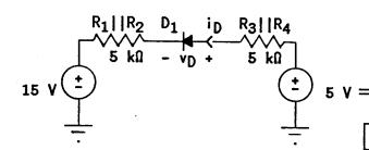
In this equivalent circuit, the voltage on the right side tends to forward bias  $D_1$ , while the voltage on the left side tends to reverse bias  $D_1$ . The latter voltage is larger, hence  $D_1$  becomes reverse biased with  $D_1 = 0$  and  $D_2 = 0$  negative. The voltage
