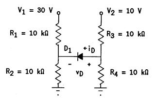
4.6 Find the diode voltage and current in the following circuit.  $D_1$  has a turn-on voltage of  $V_f = 0.5 \text{ V}$ .
