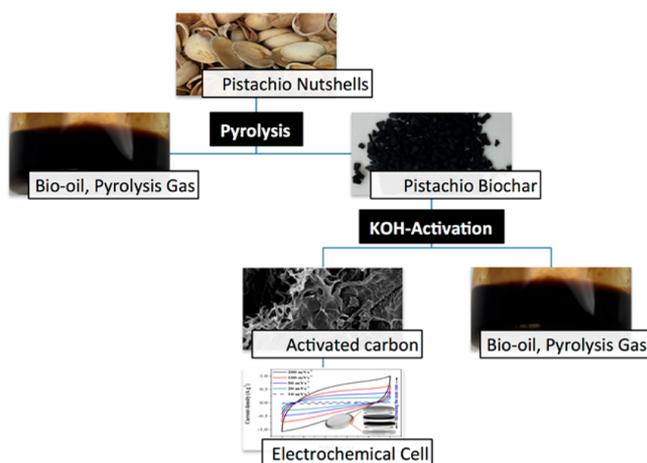
**Figure 1.** Proposed integrated process pathway for production of biofuels and electrochemical cell components from KOH-activation of biomass (i.e., activated biochars).
