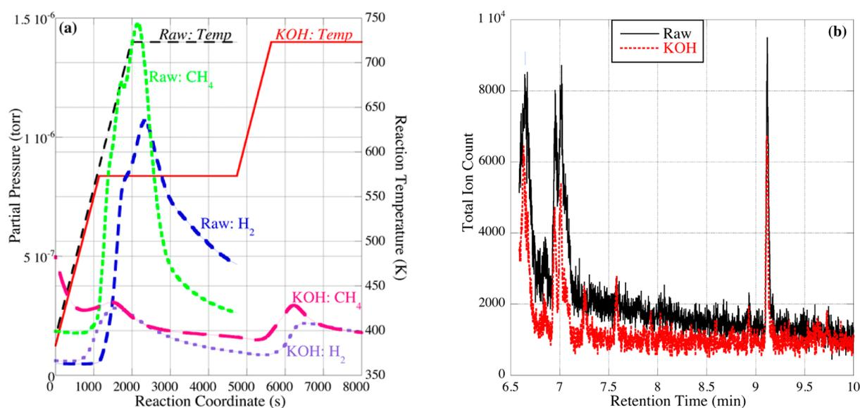
**Figure 3.** Analysis of  $H_2$  and  $CH_4$  evolved in pyrolysis gas (a) and liquid (b) biofuels produced from raw pistachio nutshells and activated biochars. (a) Pyrolysis gas evolved and monitored by MS during pyrolysis. (b) Bio-oil condensed in dichloromethane and analyzed by GC-MS after pyrolysis.
