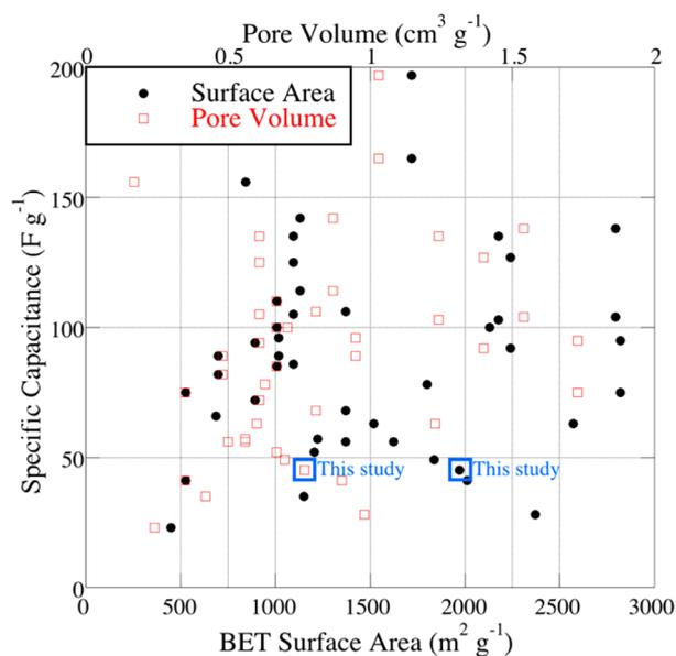
**Figure 6.** Specific capacitance as a function of BET surface area (●) and pore volume (□) for literature examples of activated-carbon supercapacitor electrodes (data compiled for this figure available in the Supporting Information).
