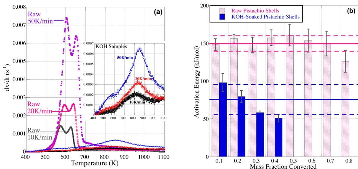
**Figure 2.** Thermal analysis of pyrolysis of raw and activated pistachio shells. (a) Derivative thermogravimetric curves for raw and KOH-activated pistachio shells pyrolyzed at 10, 20, and 50 K/min (inset magnifies KOH samples). (b) Activation energies of pyrolysis for raw and KOH-soaked pistachio shells at 10 wt % conversions from 0.1 to 0.8 (raw) and 0.1 to 0.3 (KOH); error bars indicate  $\pm$  one standard deviation; horizontal lines indicate average  $E_a \pm 1$  standard deviation).
