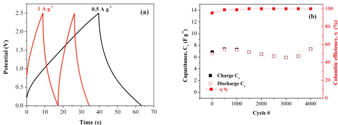
**Figure 5.** Charge–discharge studies for the supercapacitor in PC electrolyte. (a) CD curves obtained at low and high applied current densities. (b) Charge and discharge capacitance retention along with coulombic efficiency for 4000 cycles at a current density of 1 A g<sup>-1</sup>, exhibiting nearly 100% coulombic efficiency over 4000 charge–discharge performance.
