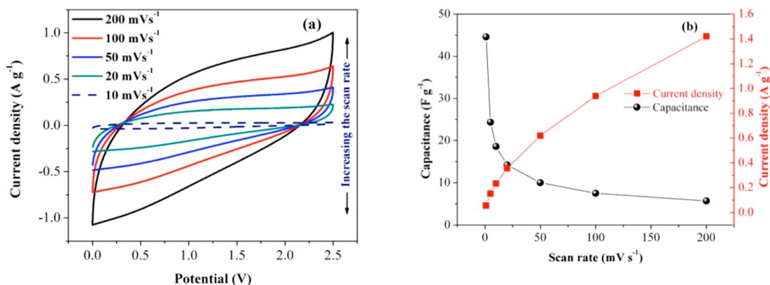
**Figure 4.** CV studies for the supercapacitor in PC electrolyte. (a) CV curves at various scan rates. (b) Calculated capacitance and corresponding current density gained at different scan rates.
