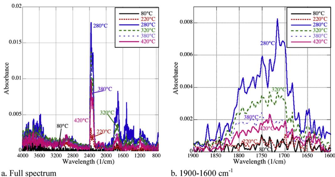
Fig. 6. Selected FTIR data for  $20\text{ }^{\circ}\text{C min}^{-1}$  pyrolysis of *D. tertiolecta* at 80, 220, 280, 320, 380 and  $420\text{ }^{\circ}\text{C}$  (3D plot and additional “snapshots” available in Supplemental Information).
