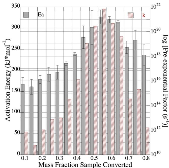
**Fig. 3.** Pyrolysis activation energy and pre-exponential factor of *D. tertiolecta* as a function of mass fraction converted (error bars indicate  $\pm$  one standard deviation).
