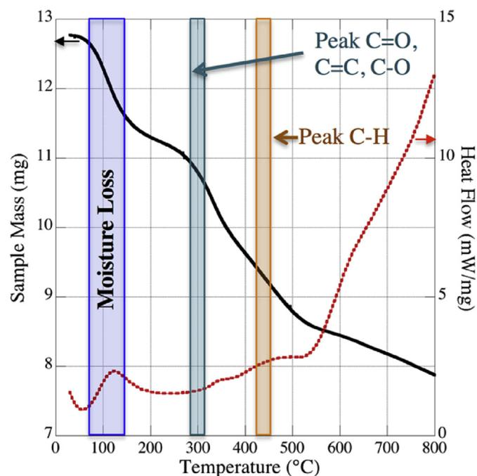
Fig. 5. TG and required heat flow curves showing primary gas evolution regions at  $20\text{ }^{\circ}\text{C/min}$  heating rate.
