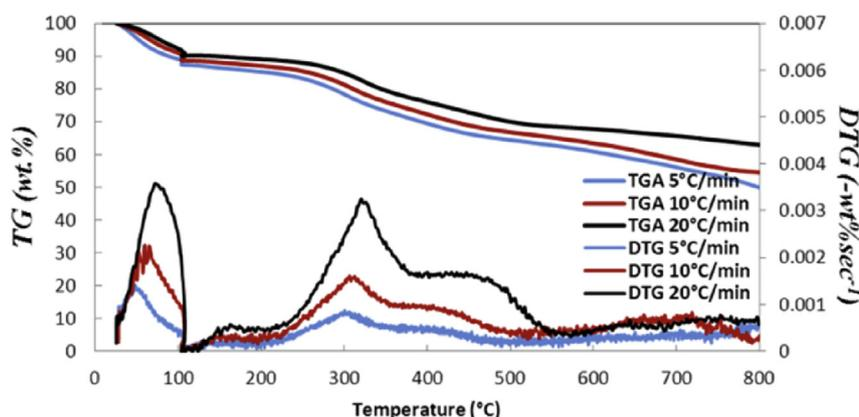
Fig. 1. Mass loss and derivative thermogravimetric curves of *D. tertiolecta* pyrolysis.
