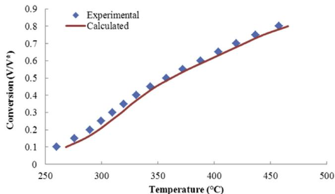
Fig. 4. Calculated (via Gaussian distribution assumption of DAEM) versus experimental data obtained for pyrolysis of *D. tertiolecta* at  $10\text{ }^{\circ}\text{C min}^{-1}$ .
