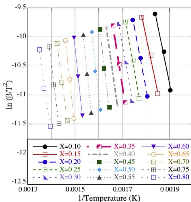
Fig. 2. DAEM plot for *D. tertiolecta* pyrolysis.
