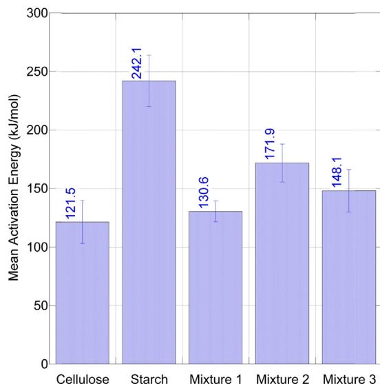
**Fig. 5.** Mean activation energy for each pure sample and blend calculated via DAEM (error bars represent 1 standard deviation).
