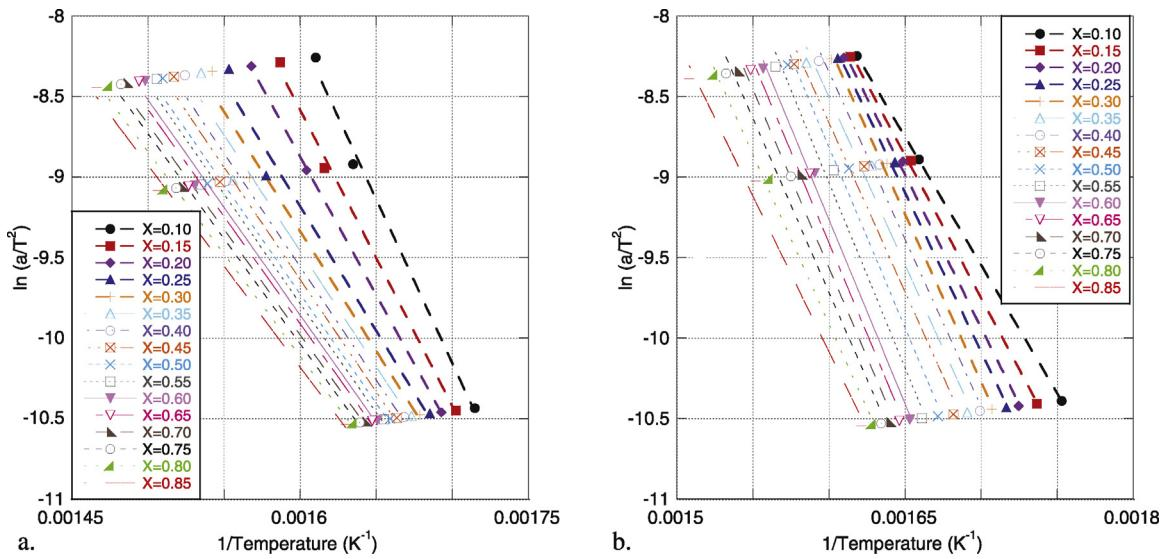
**Fig. 4.** Representative isoconversional plots for pure cellulose and 50:50 mixture at mass fractional conversions  $X = (●) 0.1; (■) 0.15; (◆) 0.20; (▲) 0.25; (+) 0.30; (△) 0.35; (○) 0.40; (□) 0.45; (□) 0.50; (□) 0.55; (▽) 0.60; (▽) 0.65; (▲) 0.70; (○) 0.75; (▲) 0.80; (—) 0.85$ .
