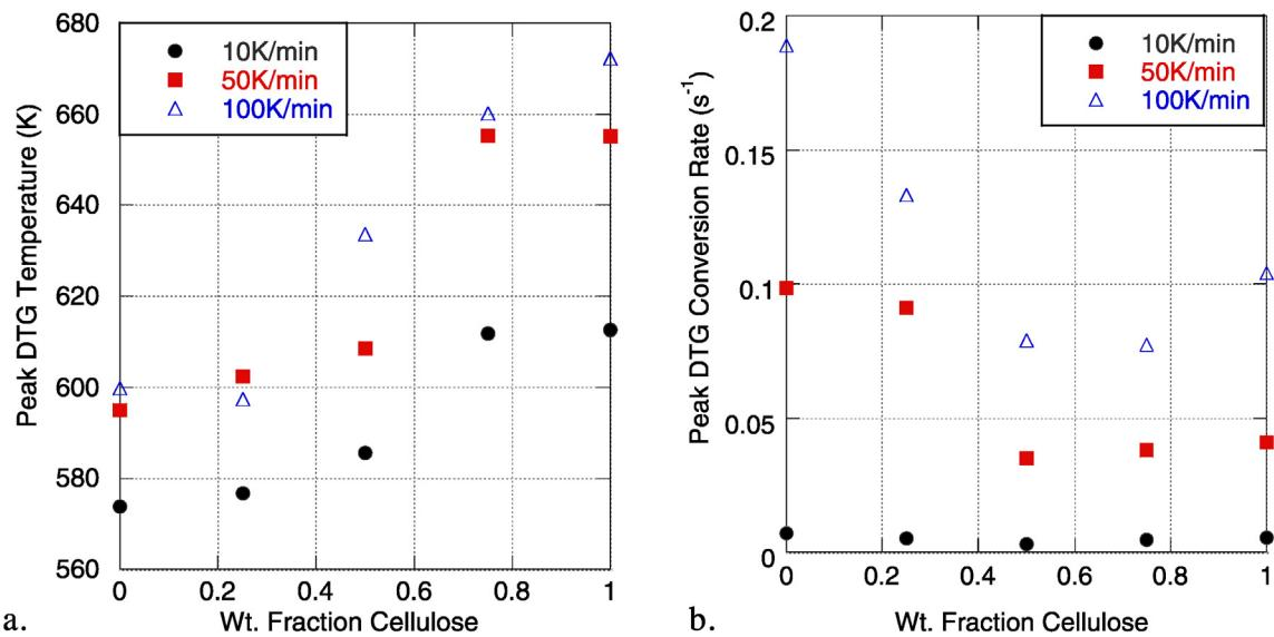
Fig. 2. Peak DTG temperature (a) and conversion rate (b) for pyrolysis of cellulose, starch and blends as a function of mass fraction cellulose at 10 K/min (●); 50 K/min (■); 100 K/min (△) (for peak 1 only).
