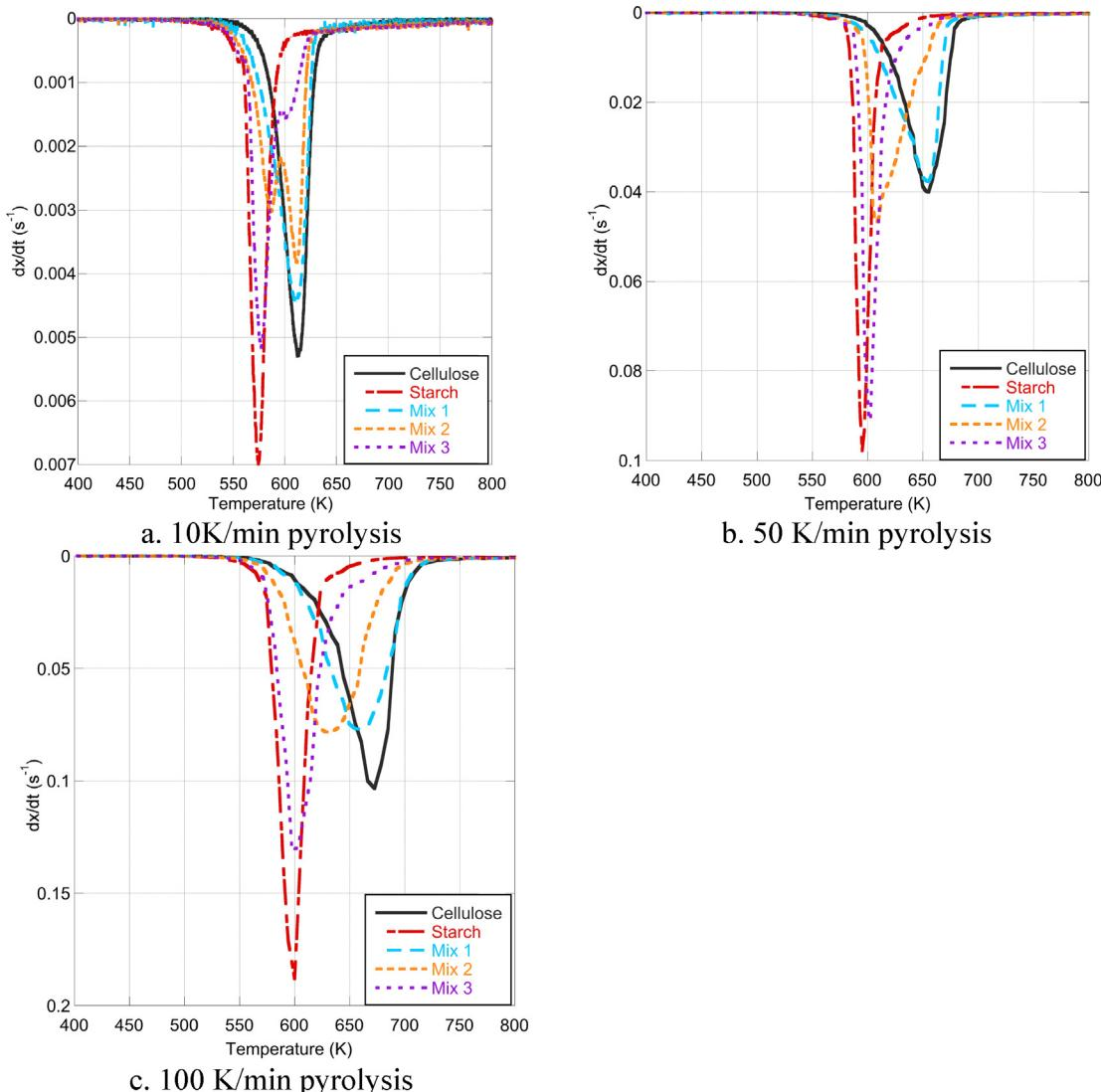
Fig. 1. Derivative thermogravimetric (DTG) curves for cellulose (—), starch (—), and blends Mixture 1: 75 wt% cellulose (—·—); Mixture 2: 50 wt% cellulose (···); Mixture 3: 25 wt% cellulose (····), pyrolyzed at 10, 50 and 100 K/min.
