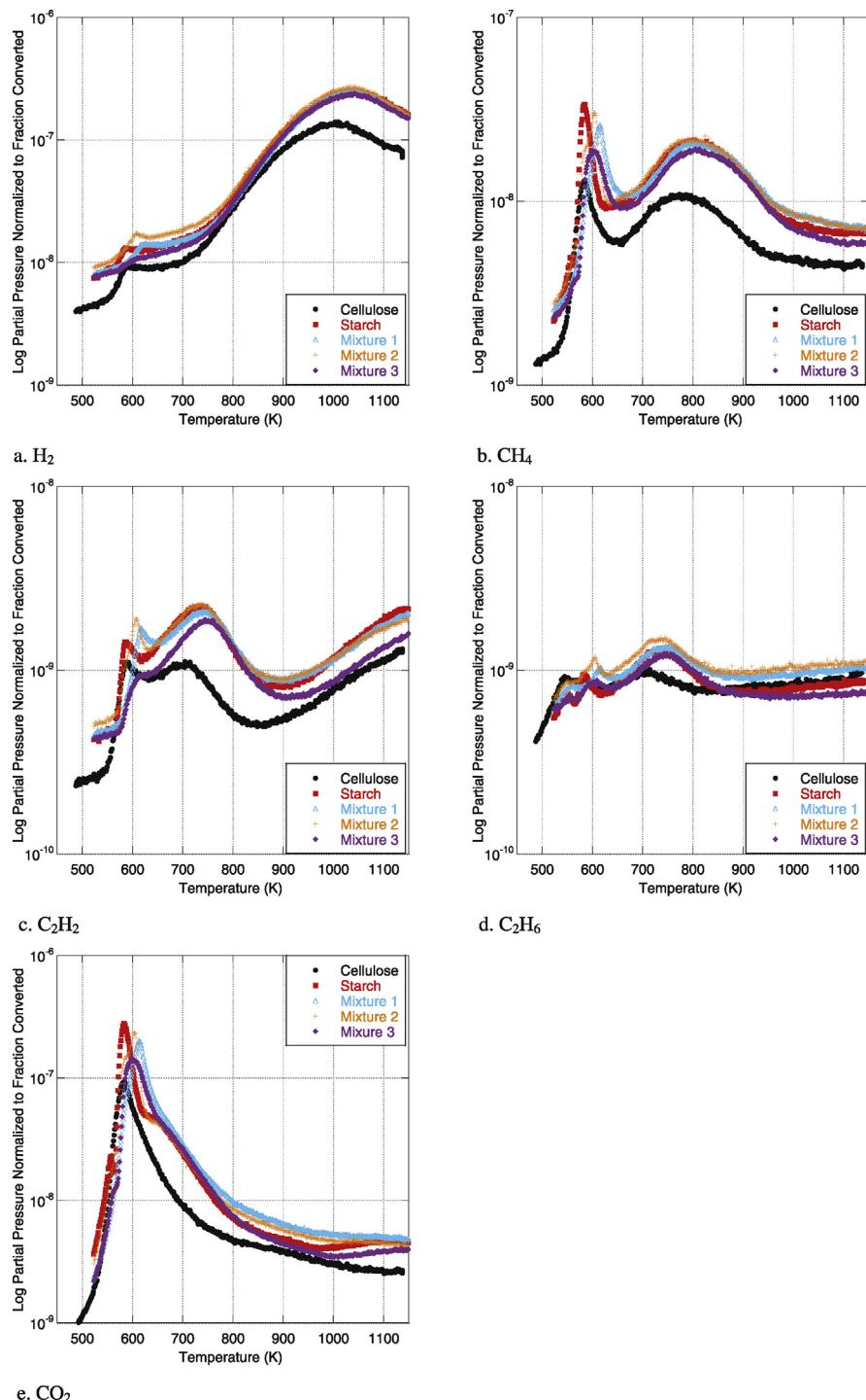
**Fig. 7.** Log of evolved gas concentrations from pyrolysis of cellulose, starch, and blends at 10 K/min for cellulose (●), starch (■), and blends Mixture 1: 75 wt% cellulose (△); Mixture 2: 50 wt% cellulose (+); Mixture 3: 25 wt% cellulose (◊). (a) H<sub>2</sub>, (b) CH<sub>4</sub>, (c) C<sub>2</sub>H<sub>2</sub>, (d) C<sub>2</sub>H<sub>6</sub> and (e) CO<sub>2</sub>.
