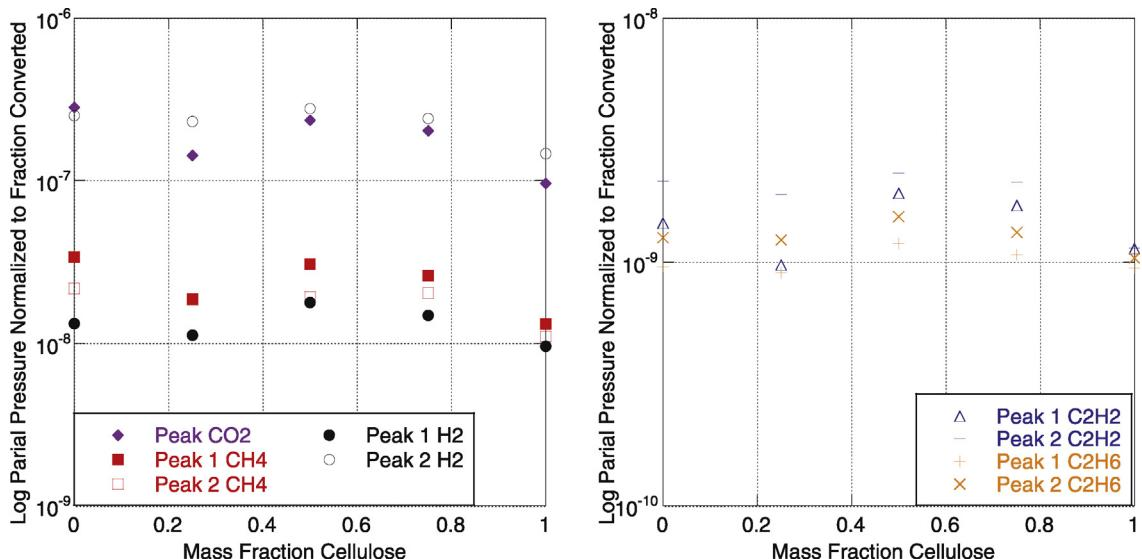
**Fig. 9.** Peak evolved gas concentration, normalized to total fraction evolved compounds as a function of mass fraction of cellulose for each pure compound and mixture pyrolyzed at 10 K/min: H<sub>2</sub> Peak 1 (●), H<sub>2</sub> Peak 2 (○), CH<sub>4</sub> Peak 1 (■), CH<sub>4</sub> Peak 2 (□), Peak CO<sub>2</sub> (◆), C<sub>2</sub>H<sub>2</sub> Peak 1 (△), C<sub>2</sub>H<sub>2</sub> Peak 2 (—), C<sub>2</sub>H<sub>6</sub> Peak 1 (+), C<sub>2</sub>H<sub>6</sub> Peak 2 (×).
