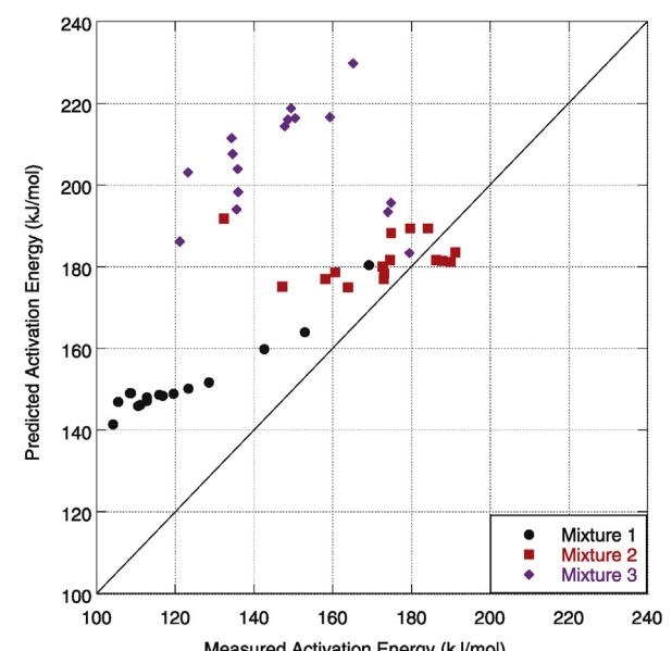
**Fig. 6.** Predicted (Eq. (4)) versus measured (DAEM) activation energy at each mass fraction conversion level for starch–cellulose mixtures.
