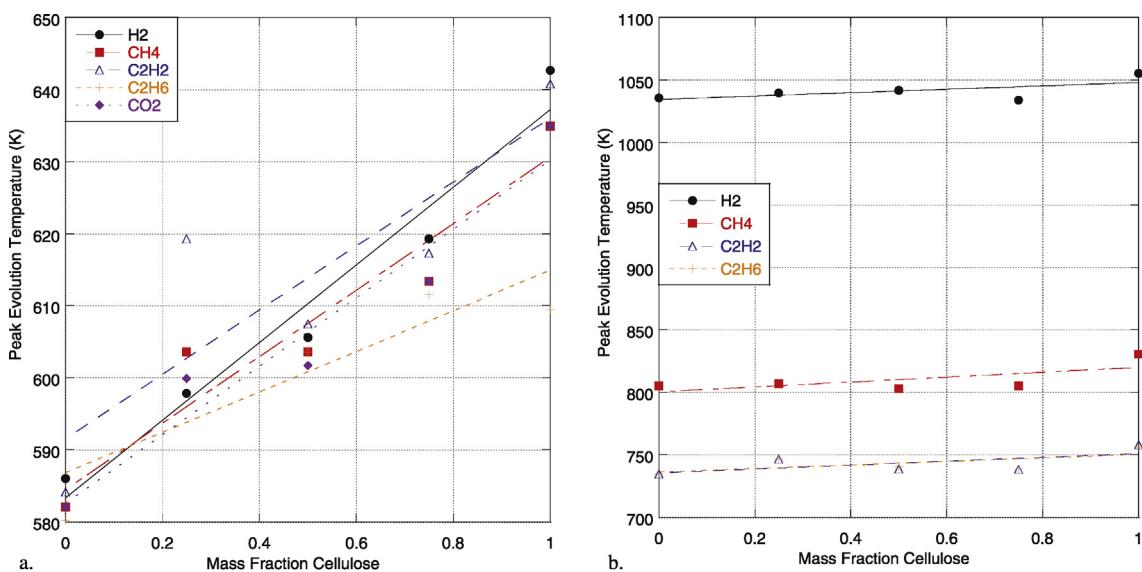
**Fig. 8.** Temperatures of peak evolution of evolved gases as a function of mass fraction of cellulose for each pure compound and mixture pyrolyzed at 10 K/min: H<sub>2</sub> (●), CH<sub>4</sub> (■), C<sub>2</sub>H<sub>2</sub> (△), C<sub>2</sub>H<sub>6</sub> (+), CO<sub>2</sub> (◆).
