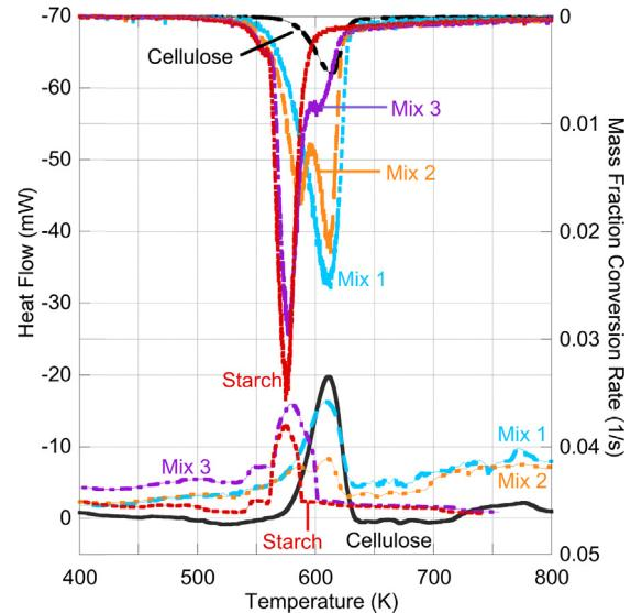
Fig. 3. Combined DTG/DSC plot for cellulose, starch and mixtures.
