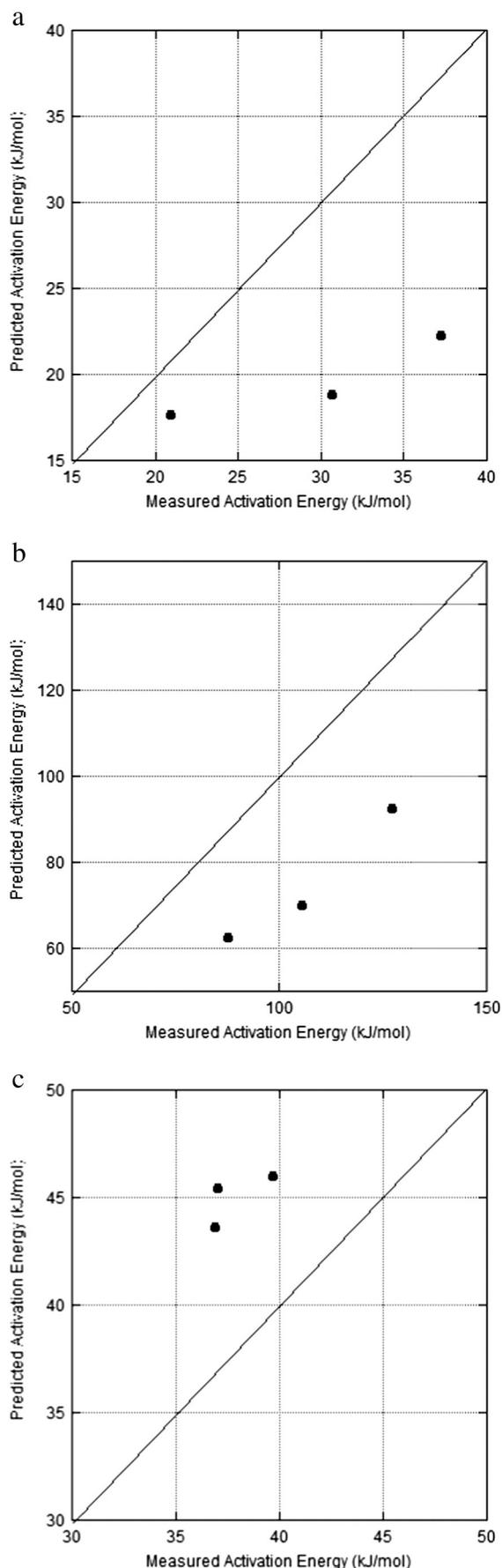
Fig. 11. Predicted activation energy of oxidation via Eq. (7) versus measured activation energy of pyrolysis for each blend for (a) mass loss regime 1; (b) mass loss regime 2; and (c) mass loss regime 3.
