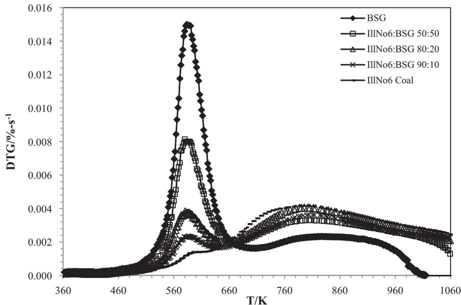
Fig. 2. DTG curves for the oxidation of BSG, Illinois No. 6 coal, and their blends at heating rate of 100 K/min.
