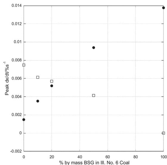
**Fig. 3.** Peak derivative mass loss rate for the pyrolysis of BSG, Illinois No. 6 coal, and their blends as a function of percent (by mass) BSG in Illinois No. 6 coal at (●) 590 K and (□) 740 K.
