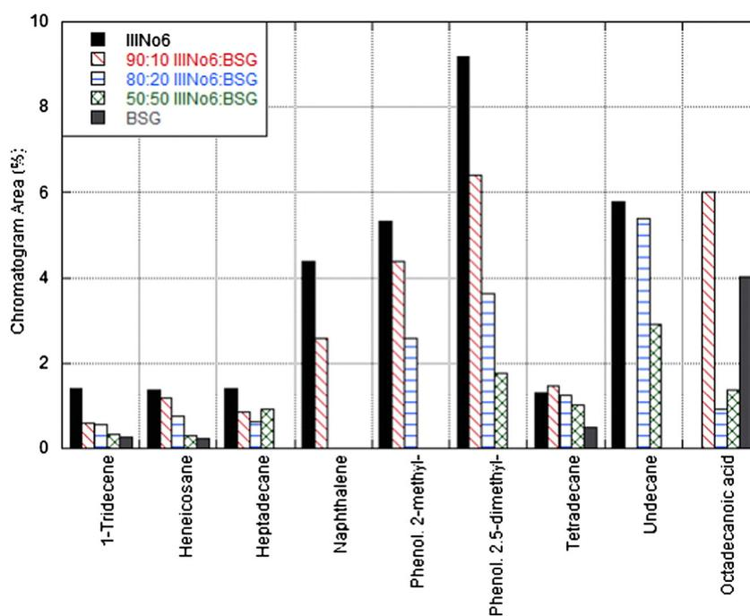
**Fig. 12.** Percent of chromatogram area of select compounds detected in rapid pyrolysis of Illinois No. 6 coal, BSG and blends at 100 °C/min (solid black = IllNo6; diagonal red = 90:10 IllNo6/BSG; horizontal blue = 80:20 IllNo6/BSG; cross-hatch green = 50:50 IllNo6/BSG; solid gray = BSG).
