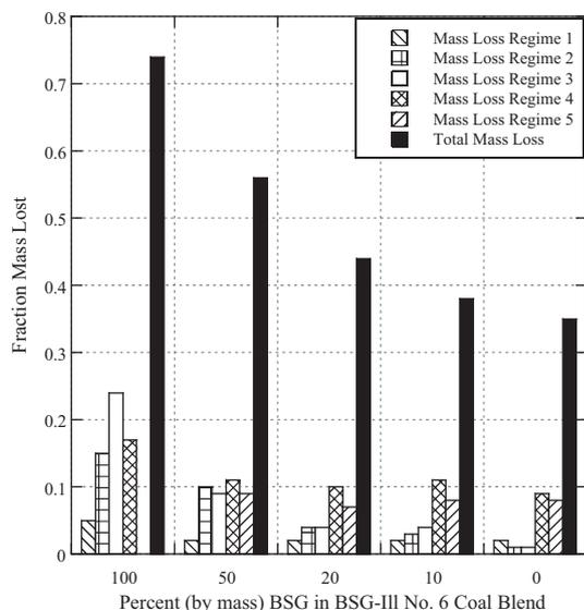
**Fig. 6.** Fraction of mass lost over each mass loss regime and fraction of total sample mass lost for each fuel and blend during pyrolysis.
