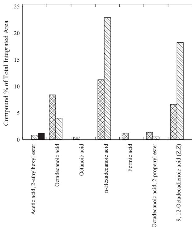
Fig. 14. Selected organic acids found during pyrolysis of BSG at heating rates of 50 °C/min (crosslinks), 100 °C/min (diagonal), and flash pyrolysis (solid).
