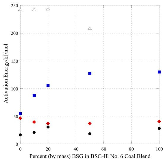
**Fig. 9.** Activation energy of oxidation as a function of percent, by mass, BSG in mixture: (●) mass loss regime 1; (■) mass loss regime 2; (◆) mass loss regime 3; (△) mass loss regime 4.
