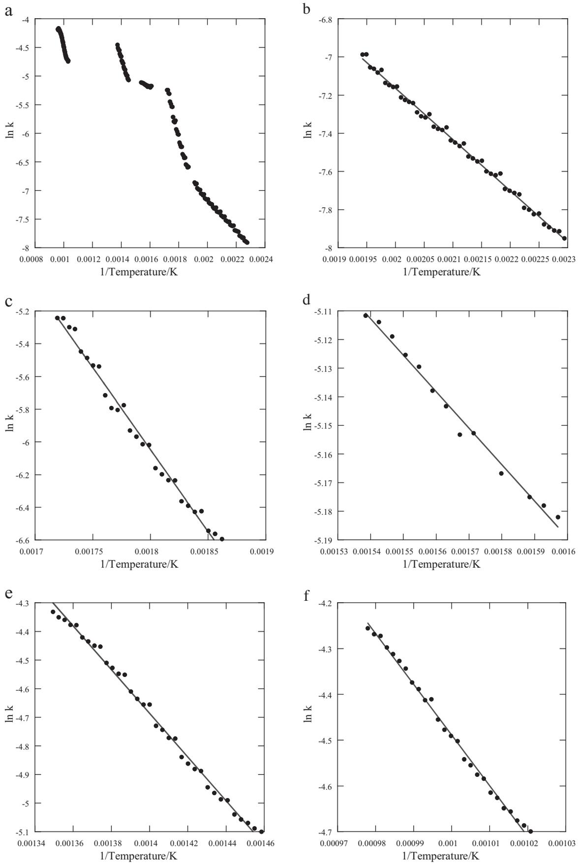
**Fig. 5.** Sample Arrhenius plot for pyrolysis of 20 wt.% BSG in Illinois No. 6 coal at 100 °C/min (a = full temperature range; b = mass loss regime 1; c = mass loss regime 2; d = mass loss regime 3; e = mass loss regime 4; f = mass loss regime 5).
