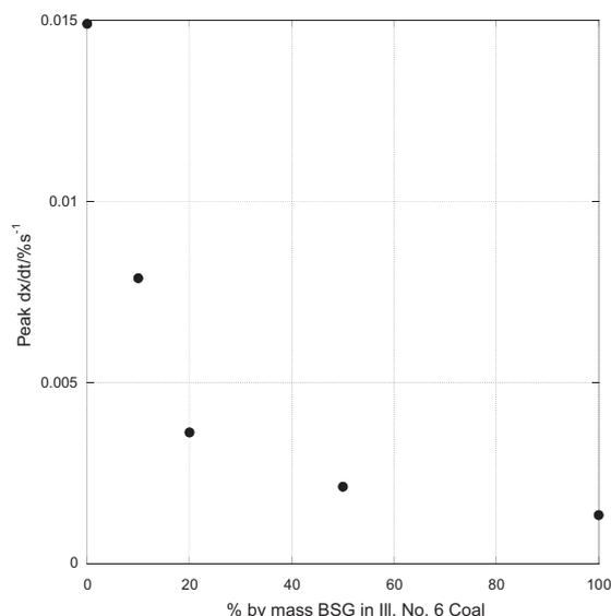
**Fig. 4.** Peak derivative mass loss rate for the oxidation of BSG, Illinois No. 6 coal, and their blends as a function of percent (by mass) BSG in Illinois No. 6 coal at 580 K.
