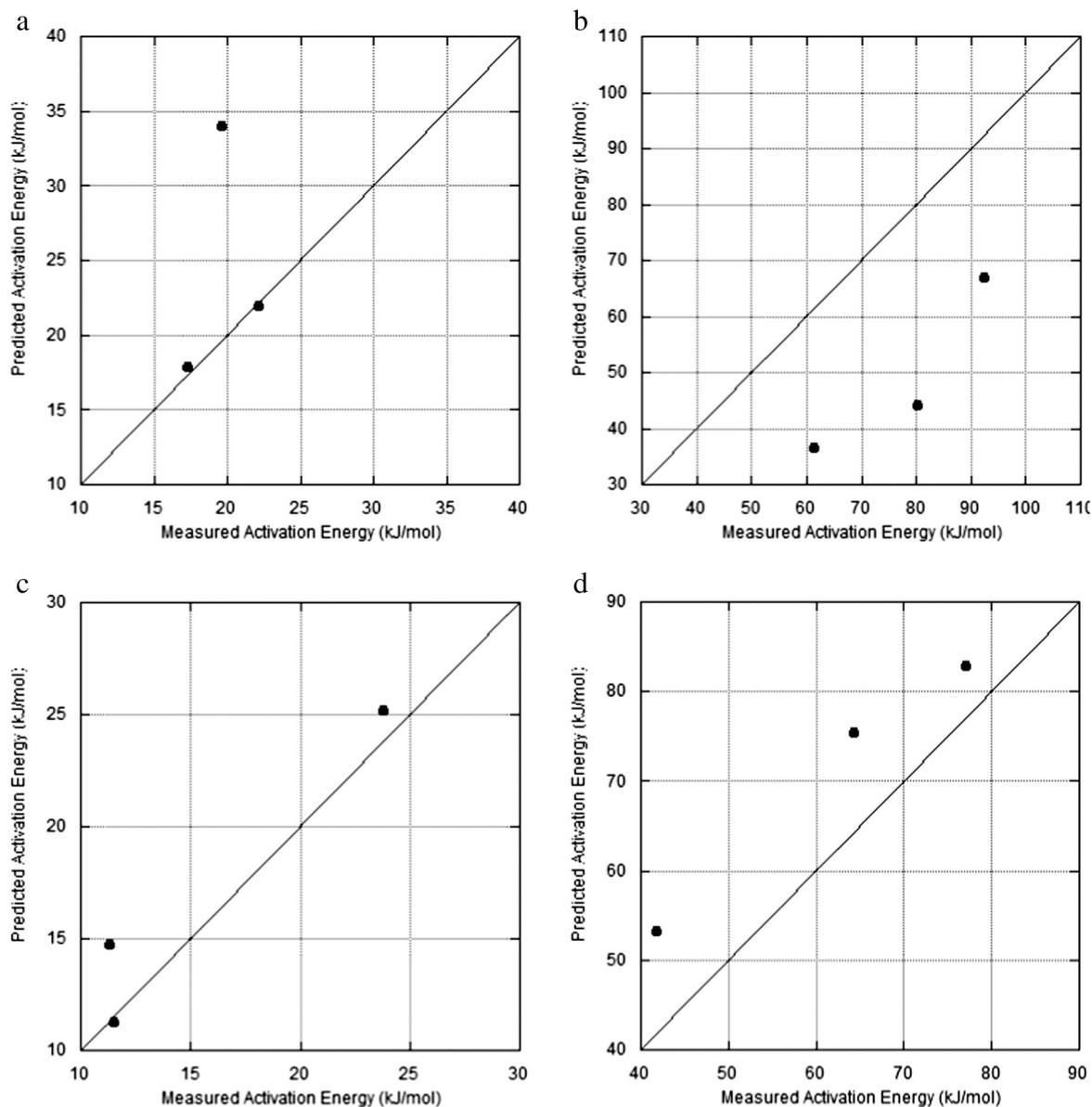
Fig. 8. Predicted activation energy of pyrolysis via Eq. (7) versus measured activation energy of pyrolysis for each blend for (a) mass loss regime 1; (b) mass loss regime 2; (c) mass loss regime 3; (d) mass loss regime 4.
