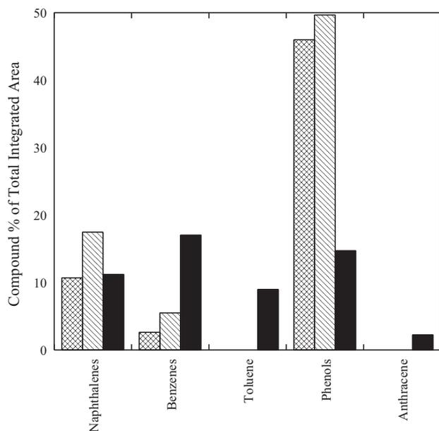
Fig. 13. Selected aromatic compounds detected in pyrolysis of IllNo6 coal at heating rates of 50 °C/min (crosslinks), 100 °C/min (diagonal), and flash pyrolysis (solid).
