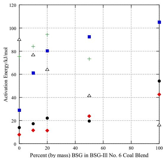
**Fig. 7.** Activation energy of pyrolysis as a function of percent, by mass, BSG in mixture (●) mass loss regime 1; (■) mass loss regime 2; (◆) mass loss regime 3; (Δ) mass loss regime 4; (+) mass loss regime 5.
