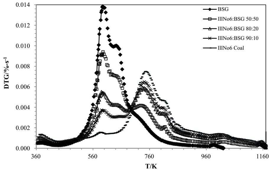
Fig. 1. DTG curves for the pyrolysis of BSG, Illinois No. 6 coal, and their blends at a heating rate of 100 K/min.
