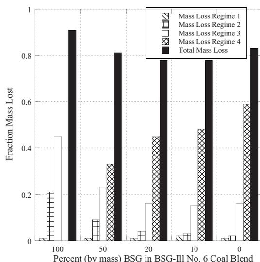
**Fig. 10.** Fraction of mass lost over each mass loss regime and fraction of total sample mass lost for each fuel and blend during oxidation.
