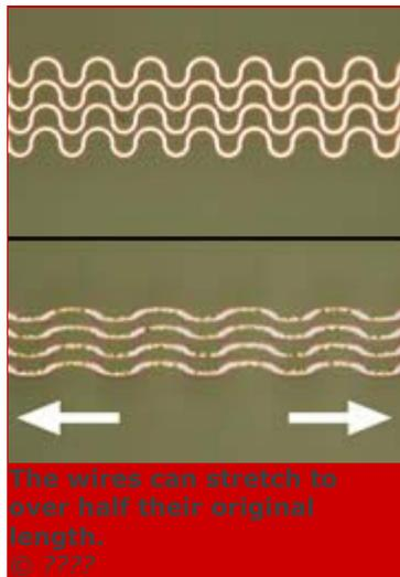
US researchers have made electronic circuits that can stretch like rubber. The flexible wires might create wearable electronics or artificial nerves that can bend inside the body.
