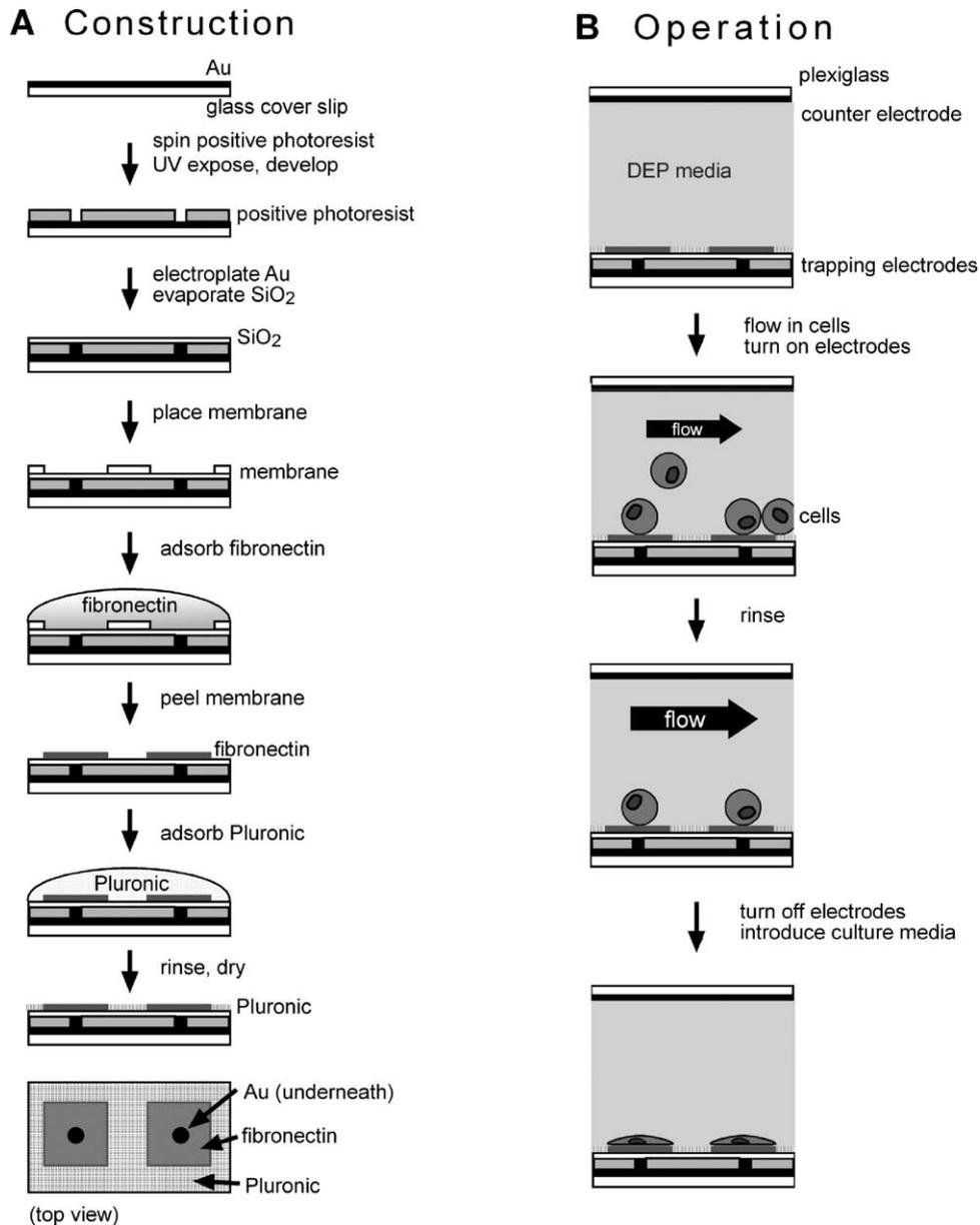
Fig. 3. (A) Construction of the DEP substrates. All views are depicted as side views; the final construction is depicted also as a top view, (B) Operation of the DEP patterning system, with substrates placed in a parallel-plate flow chamber. Construction and operation are described further in Section 2. Drawings are not to scale.
