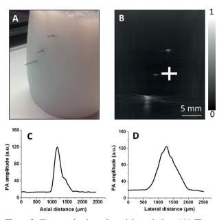
**Figure 3** Characterization of spatial resolution. (**A**) Three pencil leads were inserted into tissue-mimicking PVA gels at different depths. (**B**) Photoacoustic image of three pencil leads. The axial and lateral resolution at 19 mm depth is roughly 124  $\mu$ m (**C**) and 525  $\mu$ m (**D**), respectively.
