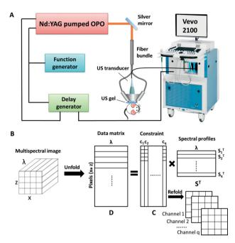
Figure 1 Schematic of the multispectral photoacoustic tomography system and the analysis method. (A) Experimental setup of multispectral photoacoustic tomography platform. (B) Flowchart of multivariate curve resolution algorithm. OPO: optical parametrical oscillator. US: ultrasound.  $\lambda$ : wavelength of the laser light. Z: imaging depth. X: imaging width.
