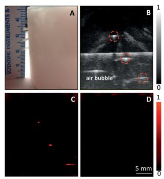
**Figure 2** Ultrasound imaging and photoacoustic tomography of a tissue-mimicking phantom with polyethylene tubes. (**A**) Three polyethylene tubes were inserted into tissue-mimicking PVA gels at different depths. (**B**) Ultrasound image of polyethylene tubes in a PVA gel, as circled. (**C**) The photoacoustic imaging depth at 1210 nm reached up to 2.7 cm. (**D**) The contrast disappeared at 1100 nm, showing that the system is bond-selective.
