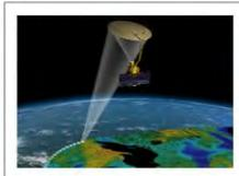
Produces real-time soil moisture observations via radio-wave backscatter
