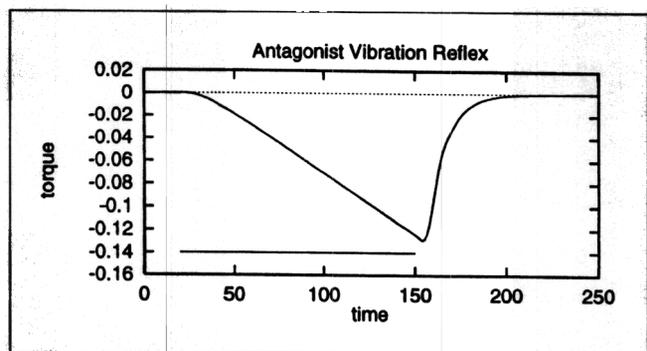
Figure 8. Simulation of the antagonist vibration reflex. Vibration was applied by setting  $vib_1 = 0.2$  during the time indicated by the horizontal line. The limb was relaxed (i.e.,  $b = 0.0$ ) and held at a position of 0.5. The solid line shows the value of the alpha motor neuron activation  $\alpha_1$ ; the reduction of this variable implies that forces are exerted into extension.
