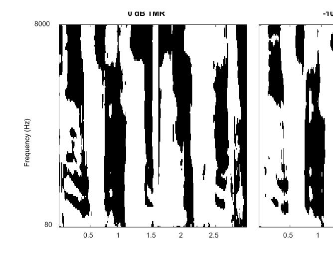
Signals were analyzed using 128 frequency channels logarithmically spaced between 80 Hz and 8 kHz, and 20ms time windows with 50% overlap.
