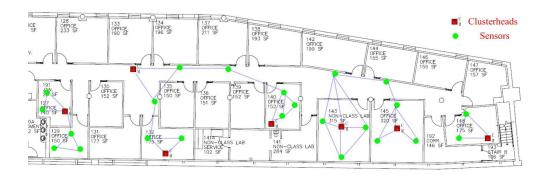
Fig. 3. Floor plan with the landmarks for the testbed.
