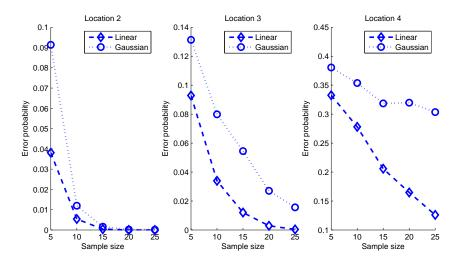
Fig. 7. Comparison of linear interpolation and the Gaussian model in terms of the error probability of GHT using the interpolated pdf.
