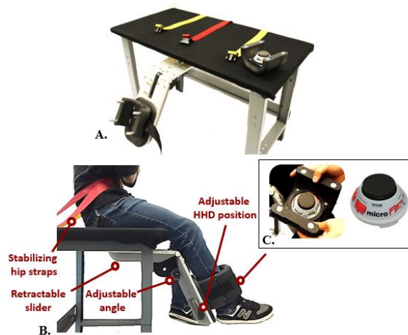
Figure 2. A) View of the device. B) Image of patient seated in the device. C) HHD housing unit.
