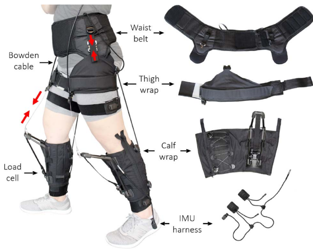
Fig. 1. Overview of the knee extension exosuit. The exosuit applies knee extension assistance by retracting a Bowden cable across the front of the knee, which is anchored to the body via a thigh wrap and a calf wrap. Additional anchoring of the thigh wrap up the side of the hip to a waist belt limits drift and also results in coupled hip abduction assistance. An inertial measurement unit (IMU) harness with load cells measures applied force and motion data.
