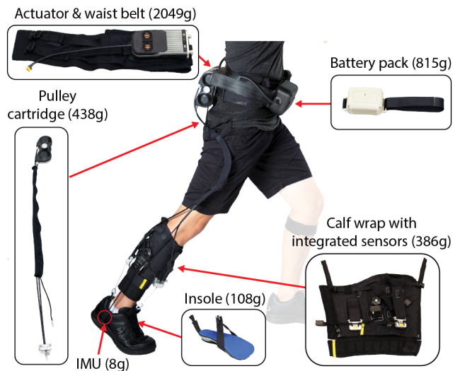
Figure 2. Exosuit hardware components and their masses
