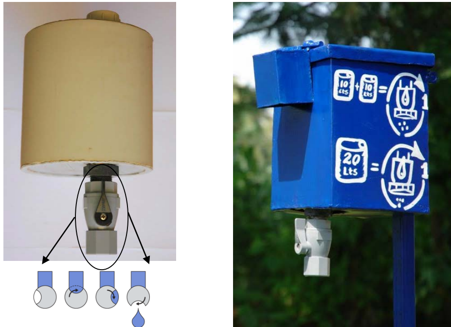
Figure 1: The Chlorine Dispenser Hardware
