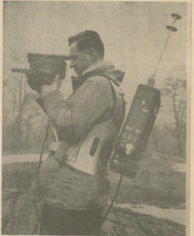
The Newschief, transistorized TV camera system produced by Sylvania Electric Products, Inc., gives cameraman increased mobility. It will be used at winter Olympics.
