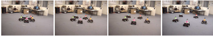
Fig. 4. Sequence of snapshots in an expansion maneuver - illustrates control of shape while pose is preserved.
