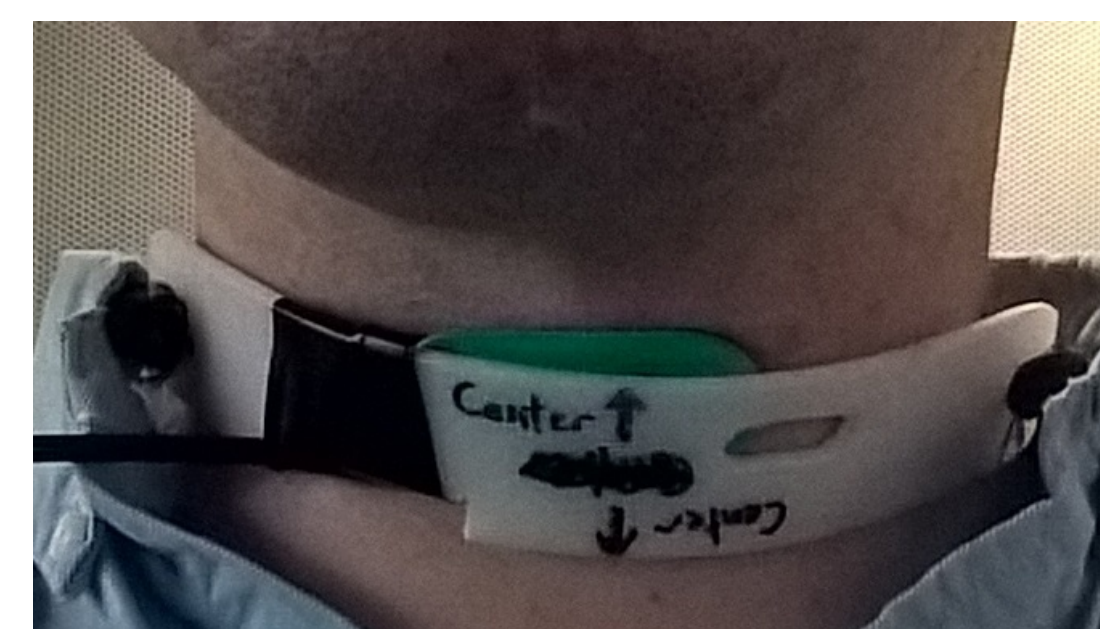
Figure 4: Laryngeal displacement device. A rigid plastic collar is fitted to a participant's neck using an elastic band. A balloon embedded in the collar is placed just under the cricoid cartilage of the larynx. During perturbation, the balloon inflates by an air tube, and pushes the cricoid cartilage dorsally and superiorly. Deflating the balloon removes the perturbation.
