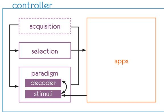
Fig. 1. A system diagram of the framework processing modules. Arrows indicate lines of communication between processing modules, handled in the background by a master controller. The effort here has been to isolate, as much as possible, the app environment from the remaining modules. This isolation is key for invoking a “crowd-sourcing” paradigm for BCI application development.
