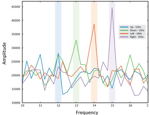
Fig. 5. Sample power spectrum during 4-choice SSVEP task.
