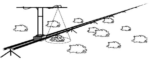
Fig. 1. A graphic display of key elements of the tram system used in the Barrow study. Tracks were leveled and supported above the ground by tripods. A cart ran along the tracks carrying the spectroradiometer. Two fiber-optic heads for the spectroradiometer were mounted on a tower attached to the cart with one head looking upward and the other looking downward at an area next to the tracks. The cart was stopped at every meter along the transect to collect a measurement.
