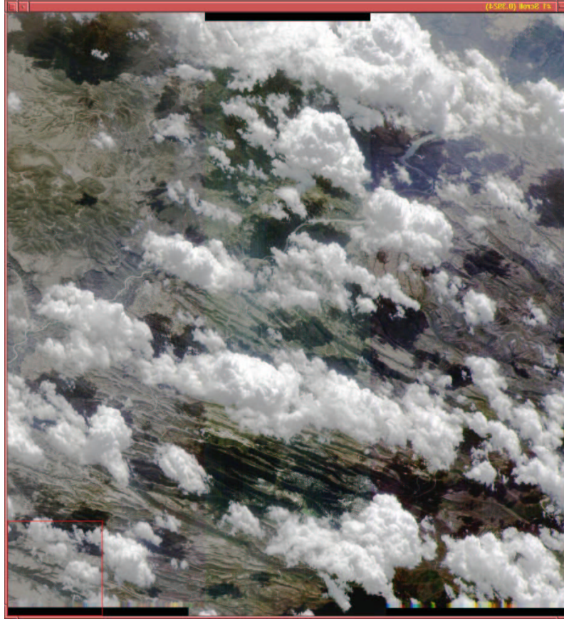
Fig. 3.17. Los Alamos (NM) scene with broken clouds captured with the Multispectral Thermal Imager (MTI) from a viewing angle of about 60^\circ . This grey-scale image was produced from a true-color rendering of the scene based on 3 narrow channels at 484, 558, 650 nm. General characteristics of the MTI instrument and orbit are given by Weber et al. (1999). For a determination of mean optical thicknesses for three selected clouds with different outer sizes, see Davis (2002).
