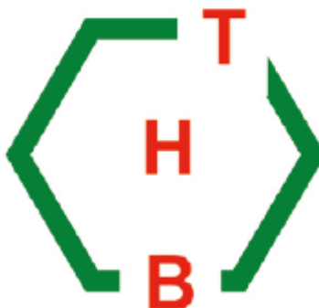
Fig. 1.24 Positions of foreign atoms on graphene: T site (top of carbon atom, also known as A site), H site (center of the hexagon), B site (bridge site). 67
